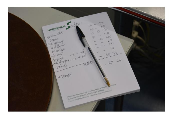
**Figure 7.** The tinting and toning values are recorded for application. The three numbers represent values of red, green, and blue light, respectively, shone through the negative to create the desired colour on the positive print.
