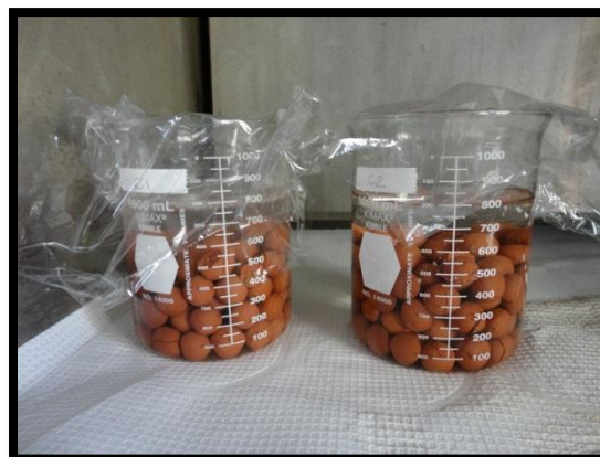
(e) Pellet soaking in conditioning brines
