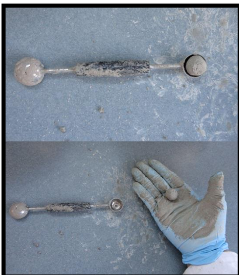
(e) Formed \frac{3}{4} inch diameter spheres with palm of hands
