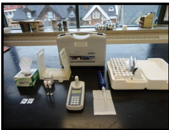
(h) MC500 Colorimeter Testing Set-Up
