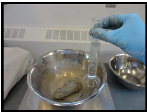
(c) Water added to workability, forming paste and kneaded
