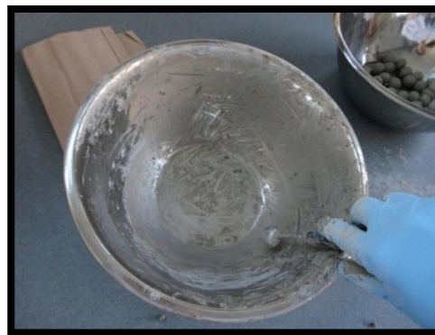
(d) Pellets extracted from paste with mellon baller
