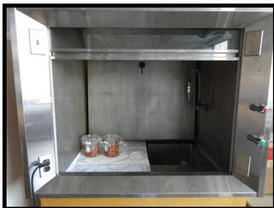
(e) Pellet soaking in conditioning brines
