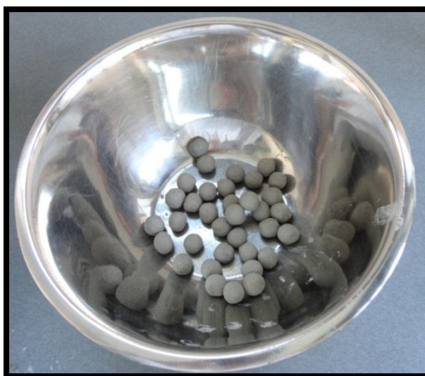
(e) Formed \frac{3}{4} inch diameter spheres with palm of hands
