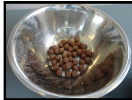
(e) Clay spheres formed as encapsulated pellets
