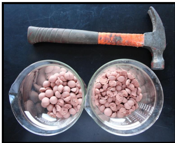
FIGURE 6.3 – PELLET SURFACE AREA DEVELOPMENT (10% LEFT AND 40% RIGHT)
