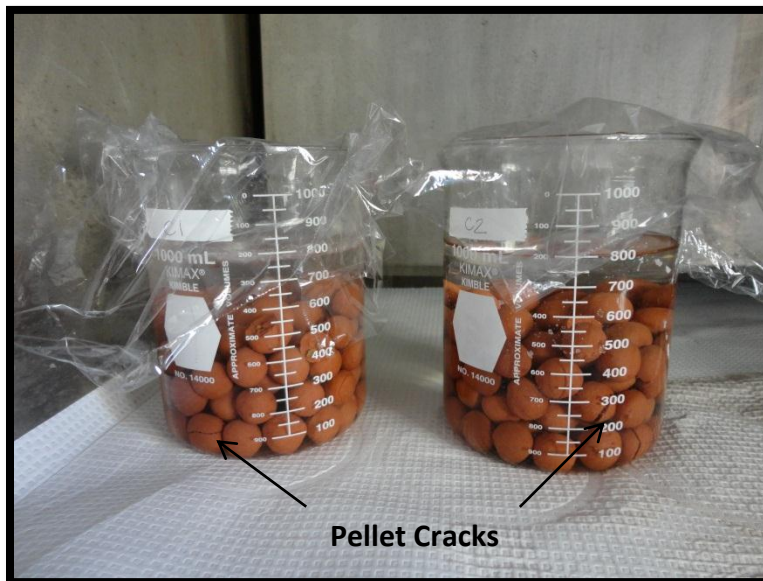
FIGURE 6.2 – PELLET TYPE 7 PHASE I CA – EXPANSION OBSERVATION
