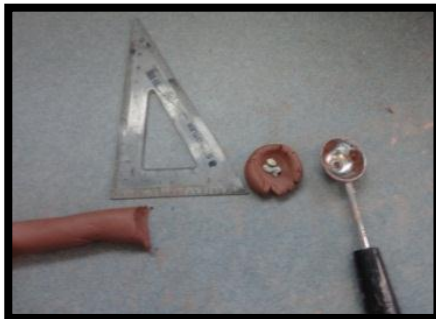
(b) Clay ball rolled out into \frac{3}{4} in diameter cylinder and clay extracted with melon baller
