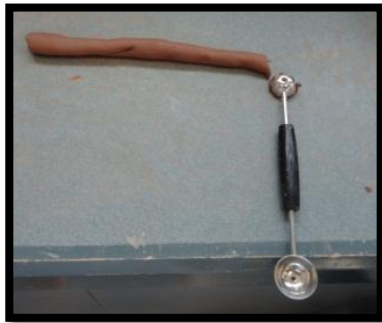
(b) Clay ball rolled out into \frac{3}{4} in diameter cylinder and clay extracted with melon baller
