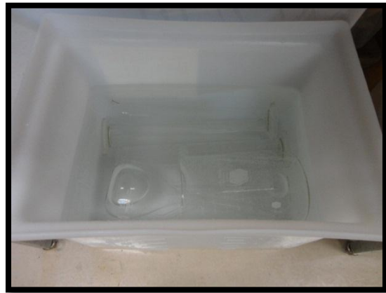
(b) Sulfuric acid bath of submerged glassware
