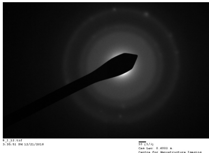
Figure 3.12 SAED pattern showing a crystalline-amorphous structure
