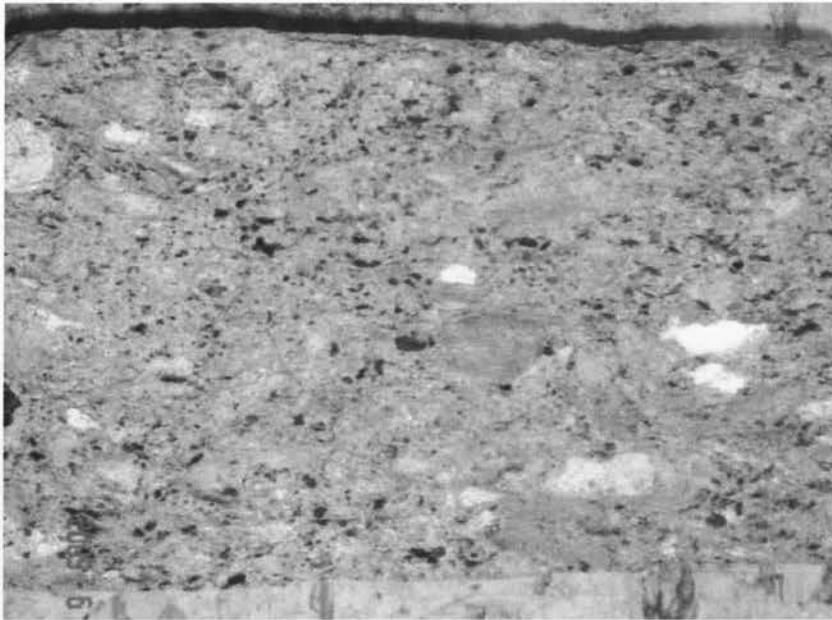
Figure 4.17: Crushed RCA2 Specimen with 8% Shingles after Indirect Tensile Test
