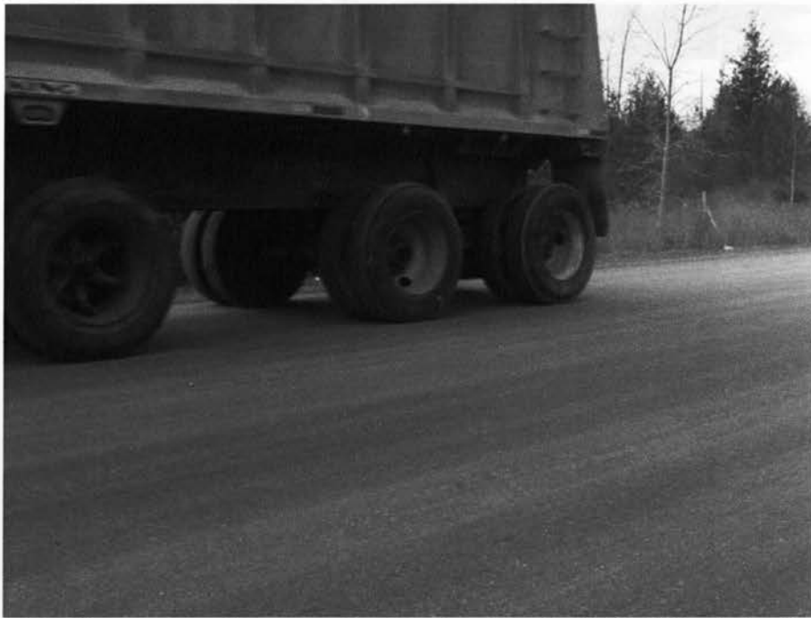
Figure 4.29: No Generation of Dust under Moving Truck (12% Shingles) after one Week
