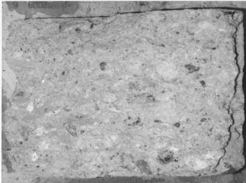
Figure 4.16: Crushed RCA2 Specimen without Shingles after Indirect Tensile Test
