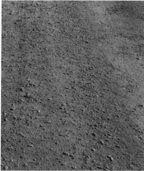
Figure 4.27: Road Surface without Shingles after one Week
