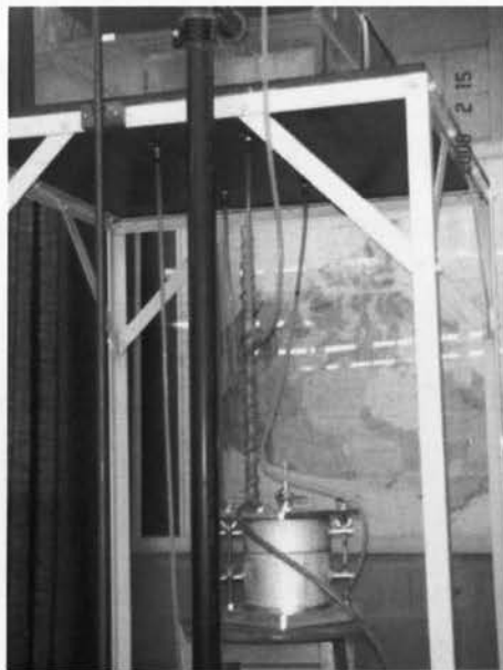
Figure 3.5: Constant Head Permeameter
