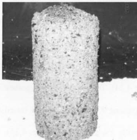
Figure 4.23: Effect of Freeze and Thaw of Fine-Sand Specimen with 10% Shingles
