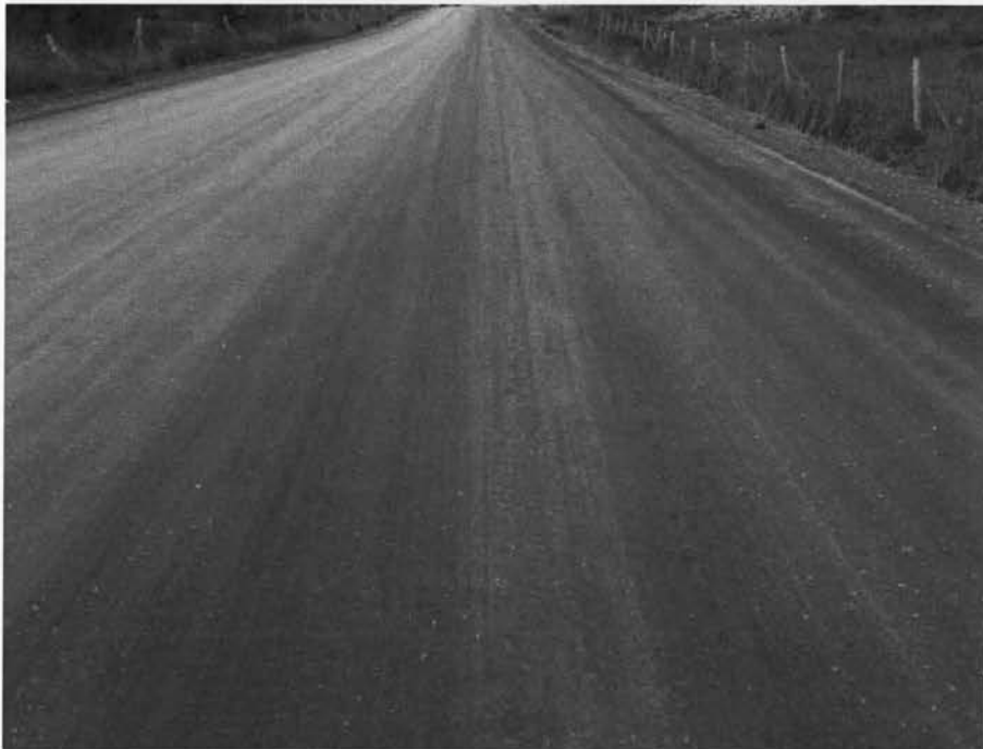
Figure 4.28: Road Surface with 12% Shingles after one Week
