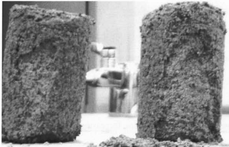
Figure 4.21: Effect of Freeze and Thaw of Fine-Sand Specimen without Shingles
