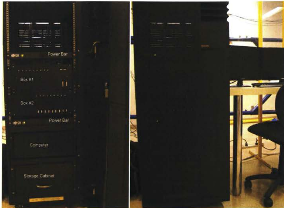
Figure 17: Rack Mounted Data Acquisition System and Workstation
