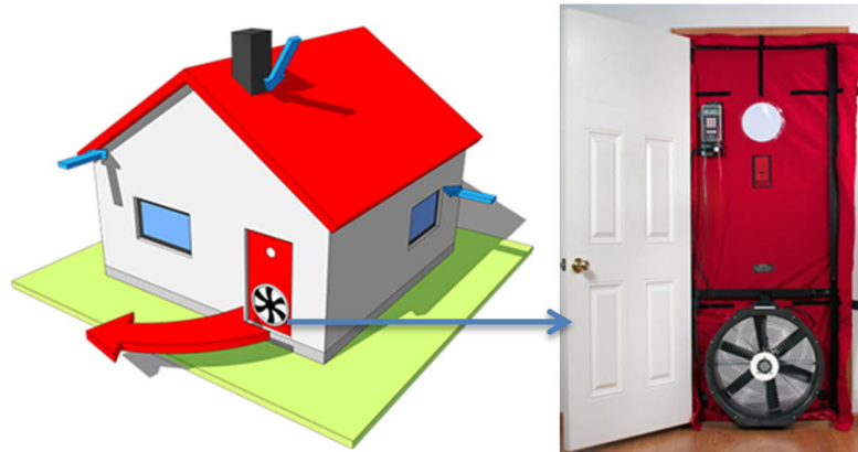
Figure 1 - Blower Door Test: left image (Lambda, 2018), right image (USI Blog, 2018)
