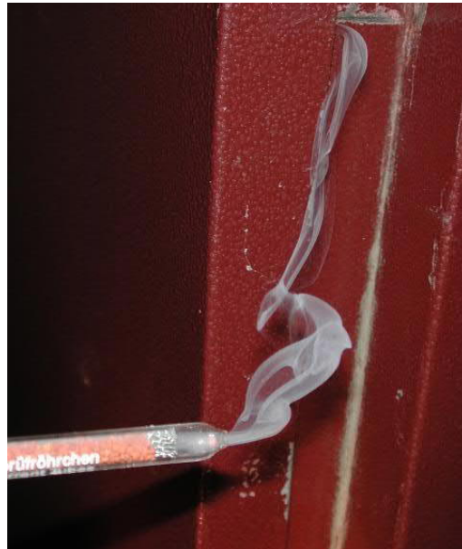
Figure 5 - Tracer Gas Method (InspectAPedia, 2017)
