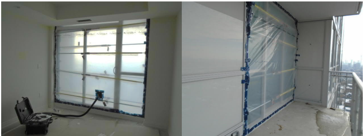
Figure 10 – Air infiltration field test through experimental window assembly set up
