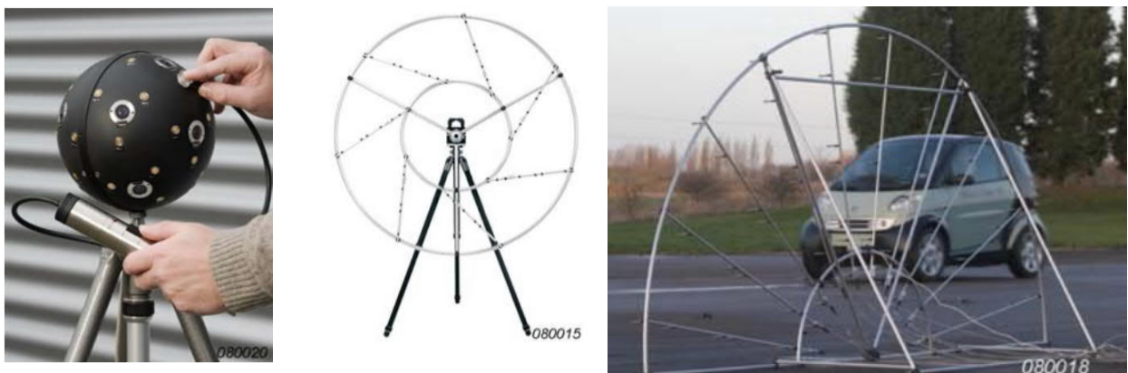
Figure 9 – Samples of microphone arrays used in beamforming technique (Briel & Kjaer, 2018)
