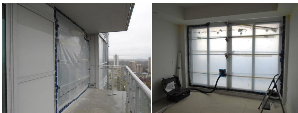
Figure 23 – Left image: Exterior view of window assembly set up, Right image: Interior view of window assembly set up of Location No. 5
