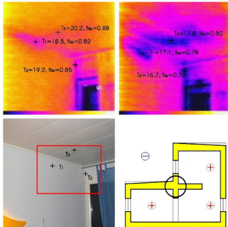
Figure 6 - Upper left: Combined building depressurization and infrared scanning, Upper right: infrared scanning (Kalamees T. , 2007)
