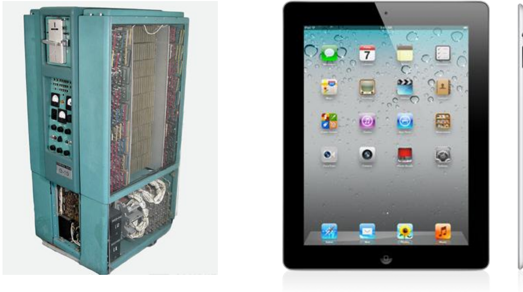
Figure 10: The G-15 from 1956 ( left ) and the magazine-sized iPad 2, 2012 ( right, show in full and profile views ). Note the accessibility of the inner parts of the G-15, and the sealed casing of the iPad 2. The iPad 2's tagline was the rather cryptic slogan: "Brilliant from the outside in," which seems peculiar given that the minimization of the iPad's "in."
