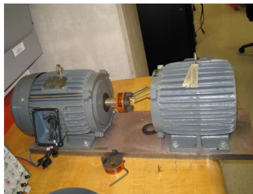
Figure (4.1) Induction motor–generator setup.
