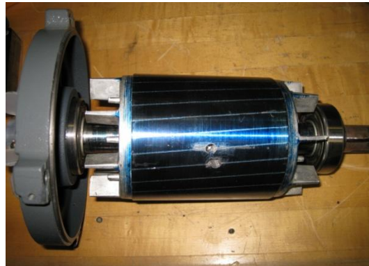
Figure (4.2) Faulty induction motor with a fabricated hole on the rotor bar
