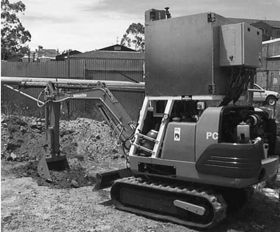
Figure 1.1: The robotic excavator developed by the ACFR in a trench forming task; from Ha et al., 2002.
