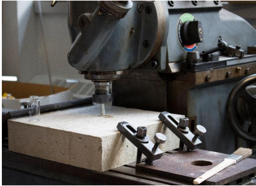
Figure 3.1-4: Slab secured to milling machine for surface grinding.
