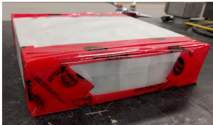
Figure 3.1-2: Concrete slab in wrapped curing condition.
