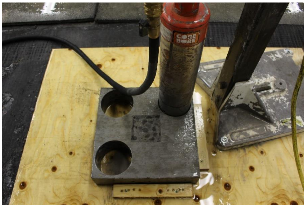
Figure 3.1-7: Slab coring setup.
