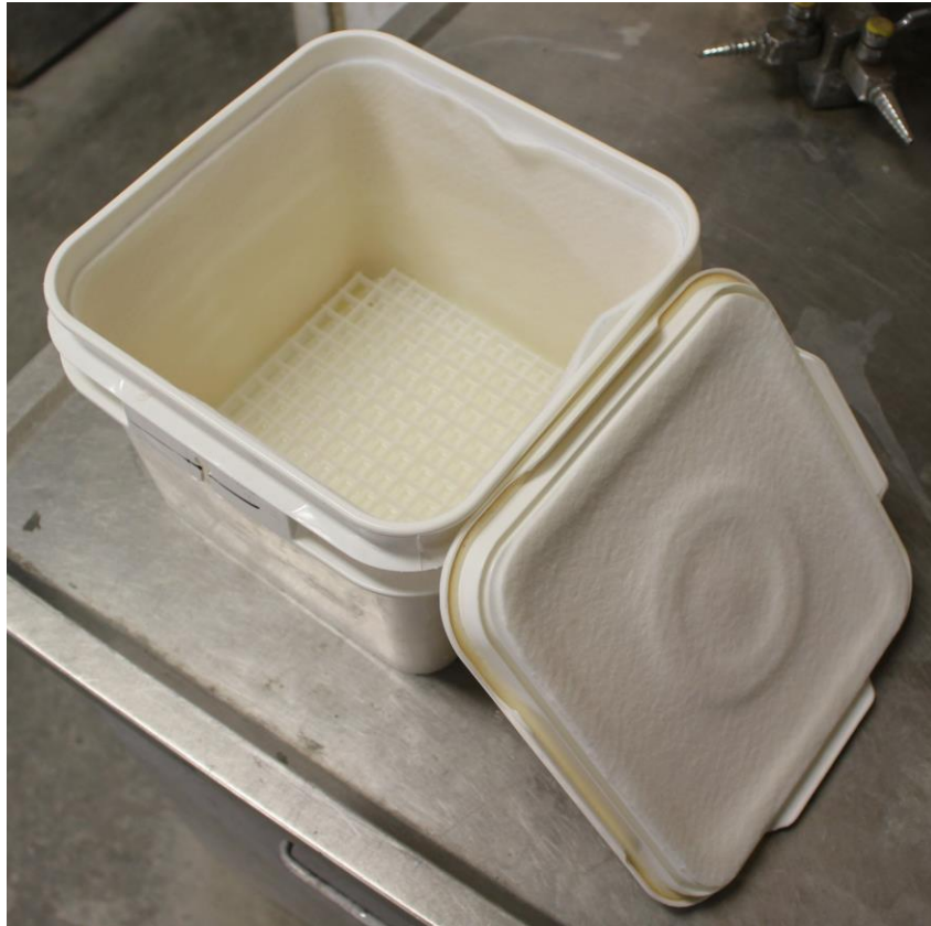
Figure 3.2-8: 150 mm cube mould storage containers for 60°C storage temperature.
