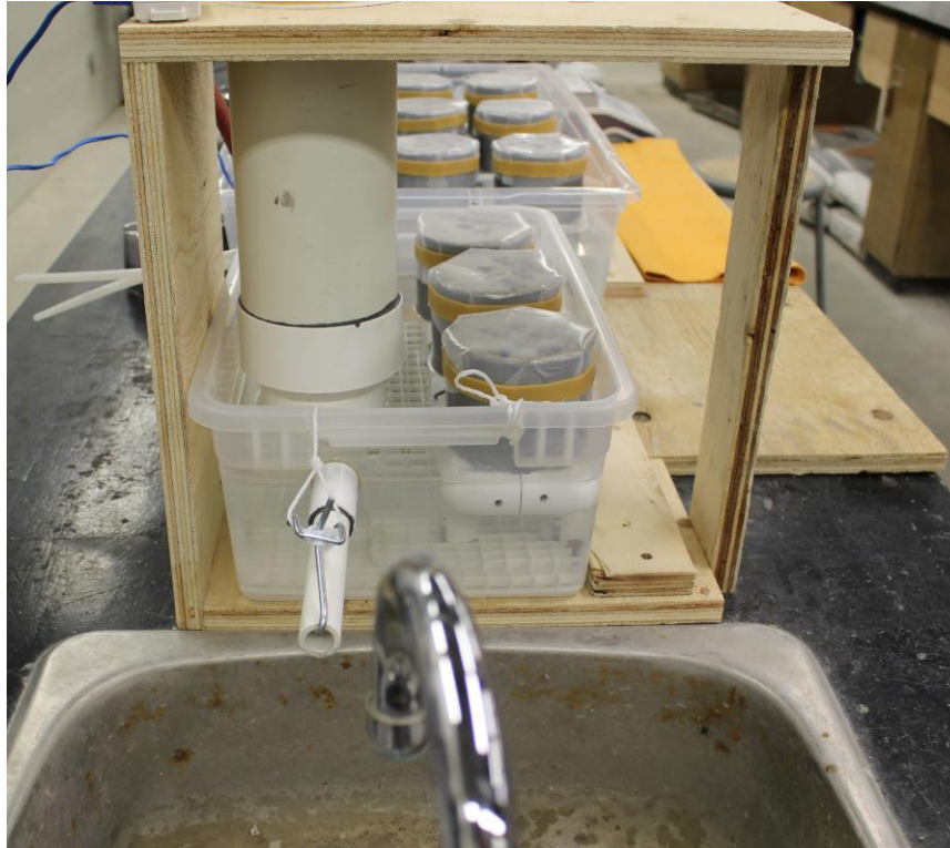
Figure 3.1-8: Apparatus for sorptivity testing.
