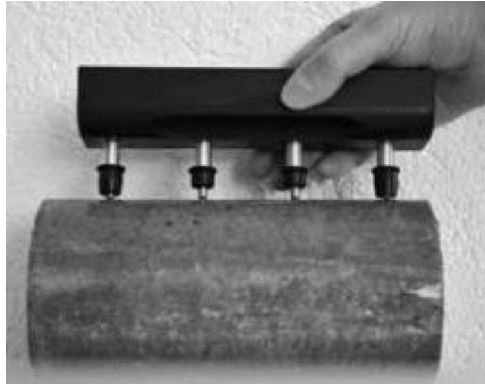
Figure 3.1-9: 4-point Wenner probe
