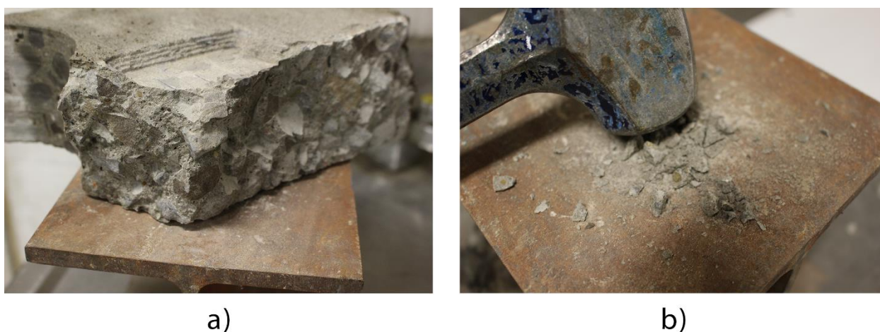
Figure 3.1-6: a) Slab with midpoint exposed; b) Pulverization of material chiseled from midpoint of slab.
