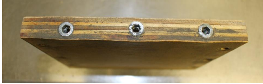
Figure 3.2-3: Tapping threads secured in edge of mould section.
