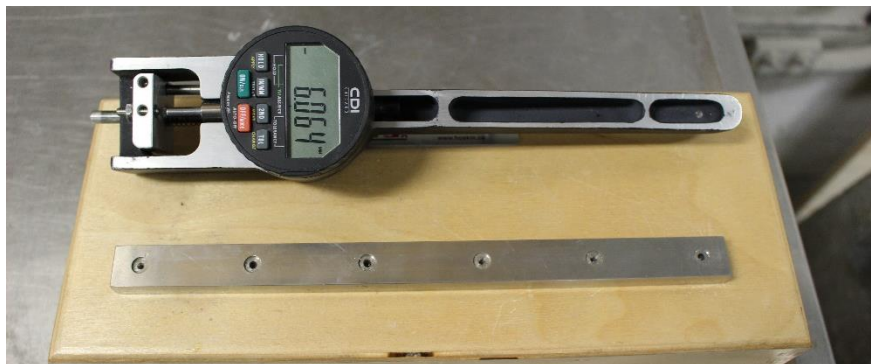
Figure 3.2-10: Variable length digital strain gauge.
