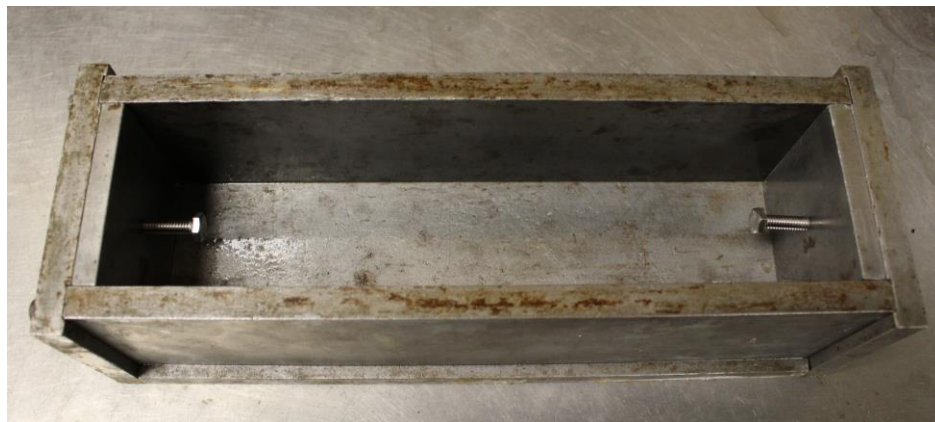
Figure 3.2-5: Metal prism moulds.
