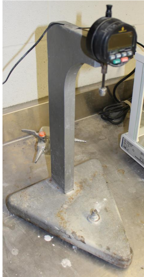
Figure 3.2-13: Length comparator apparatus used for expansion measurements of prism and cylinder specimens
