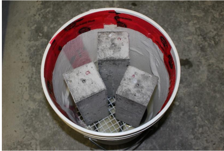
Figure 3.2-9: Prism and cylinder storage container.
