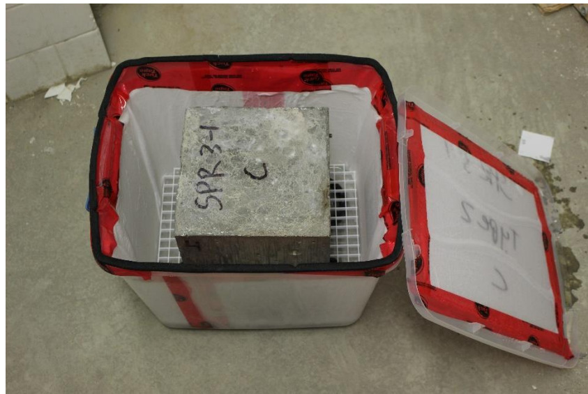
Figure 3.2-7: 150 mm and 200 mm cube mould storage containers for 38°C storage temperature.
