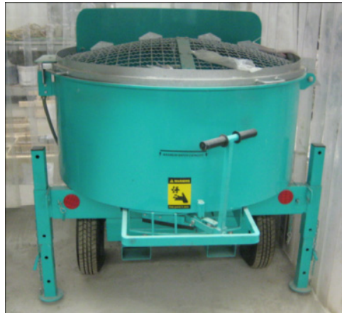
Figure 3.9: IMER Mortarman 750 vertical shaft mixer
