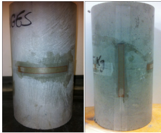
Figure 3.3: Horizontal and vertical strain gauges attached to cylinder specimen
