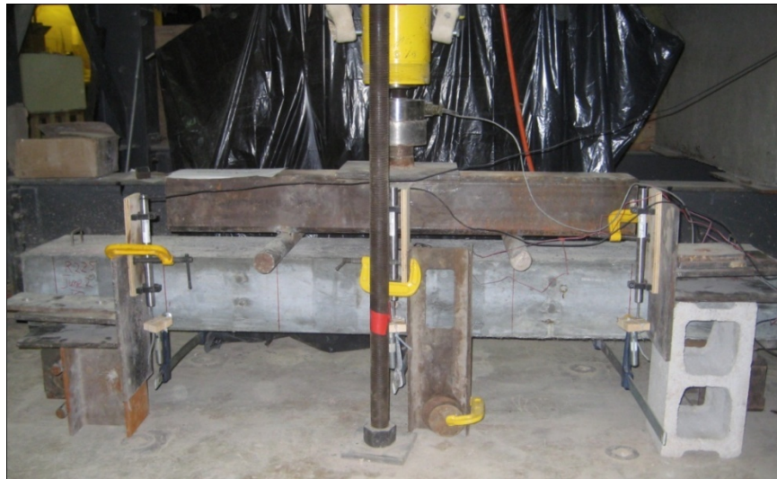
Figure 3.20: Static slab/beam test setup
