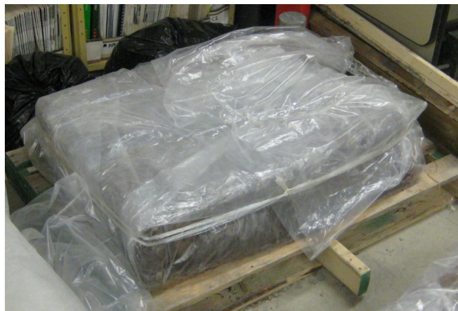
Figure 3.11: Precast slab/beams under moisture barrier and wet burlap
