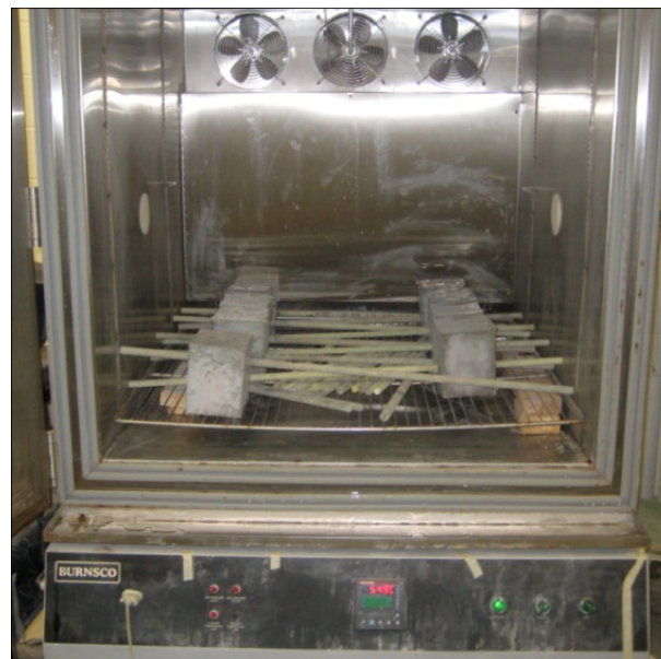
Figure 3.24: Environmental chamber for freeze/thaw application
