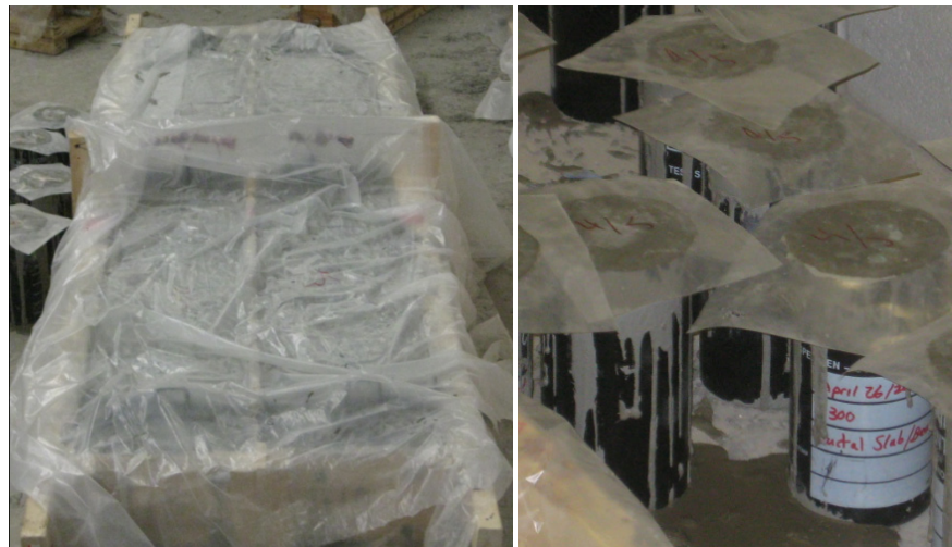
Figure 3.10: Full cast type D slab/beam specimen under plastic sheets (left) and control cylinder specimens under plastic sheets (right)
