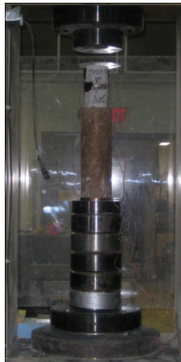
Figure 3.4: MTS setup for testing modulus of elasticity of concrete
