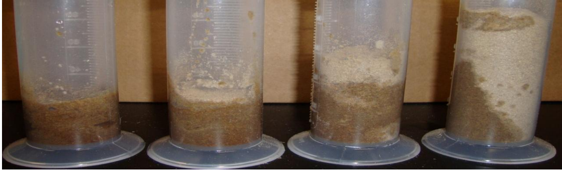
Figure 4.1 Oats straw suspensions of mesh size 60 and concentrations of 5, 10, 20 and 40 wt % made by dispersion.
