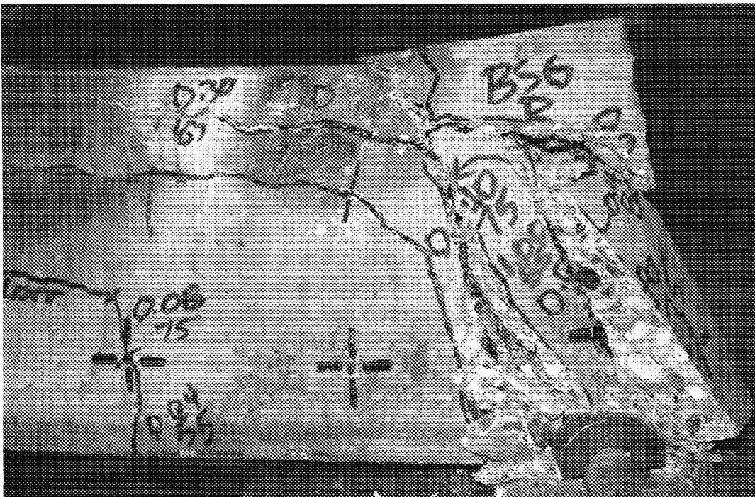
Figure E-6: Photograph showing the failure zone of BS06
