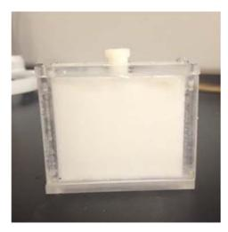
Figure A-1. Bone-mimicking phantom mould containing HA and gelatine.
