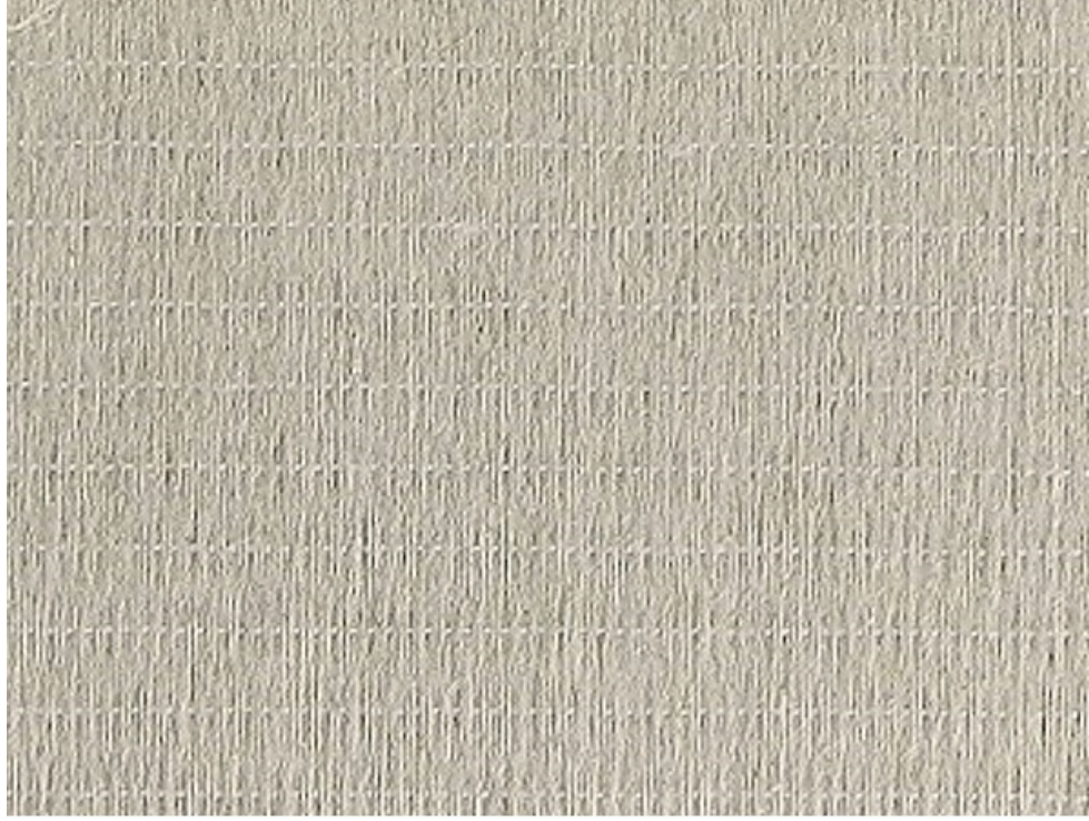
Figure 3.1: UD FlaxPly ® fabric roll from Lineo NV, Belgium, shown prepared for cutting on a flat table.
