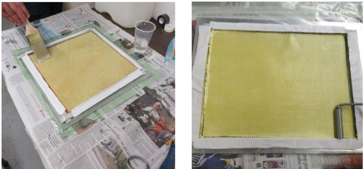
Figure 3.7: Using a laminate brush to spread resin ( left ), Using a roller to compress plies and extract trapped air ( right )
