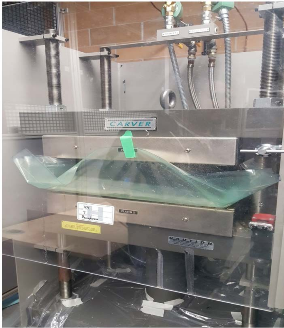
Figure 3.8: Plate assembly vacuum sealed in High temperature plastic membrane bag, and inserted in to Carver Press
