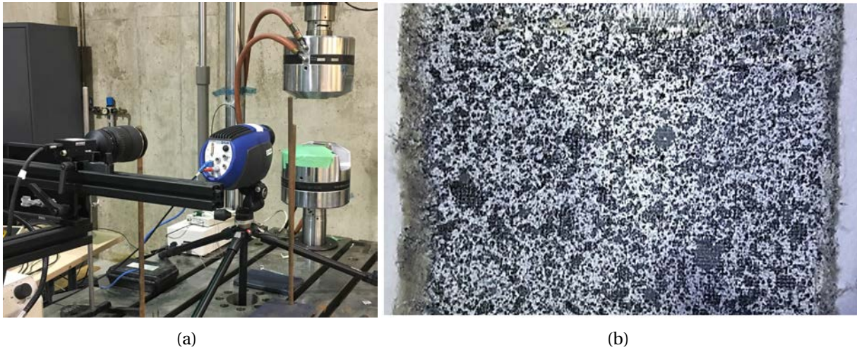
Figure 4.1: (a) Digital Image Correlation Imaging setup alongside the Testing Frame, (b) Speckled pattern sprayed on the surface of the sample
