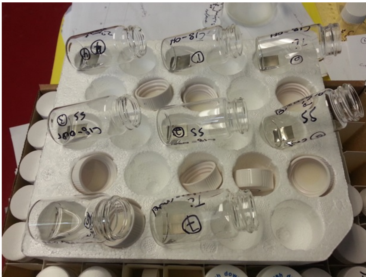
Figure 2.49: Metal coating experimental set up using 20 mL glass screw cap vial open to air.
