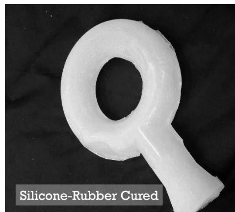
Figure 6: Silicone-Rubber Cured Cervix from 3D printed mold
