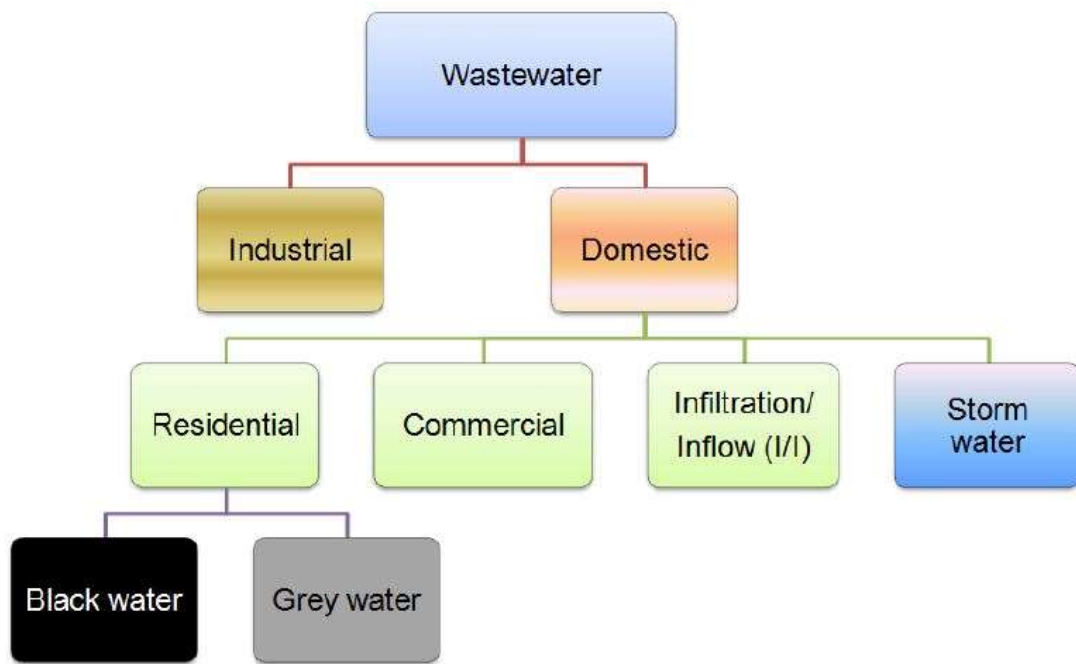
Figure 2: Typical Components of Wastewater Flow from Community (Elbeshbishy, 2016)
