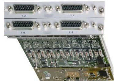
Figure 3-10 DSub-15s Connected to the CRONOS-PL unit (Left) and UNI2-8 eight-channel amplifier (Right)
