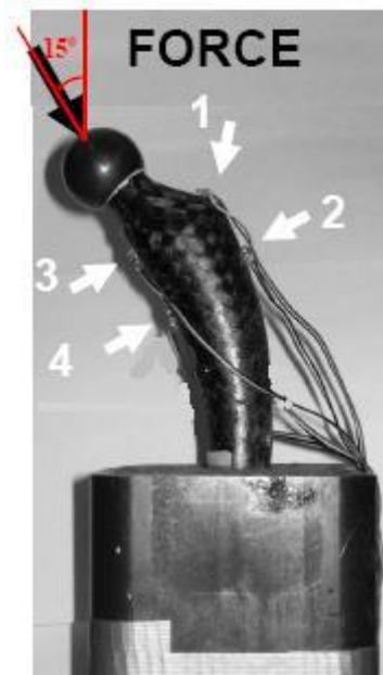
Figure 3-11 Strain gauge locations with virtual force on femoral head
