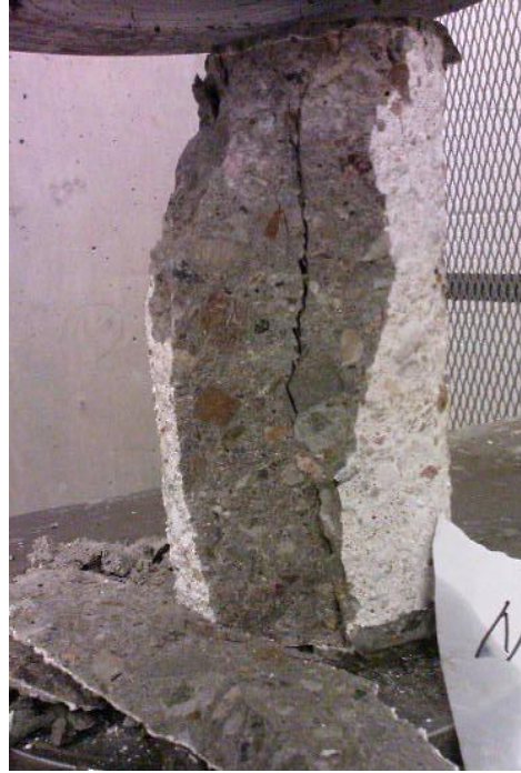
Figure 4.6 Crushed degraded concrete sample under compressive load.
