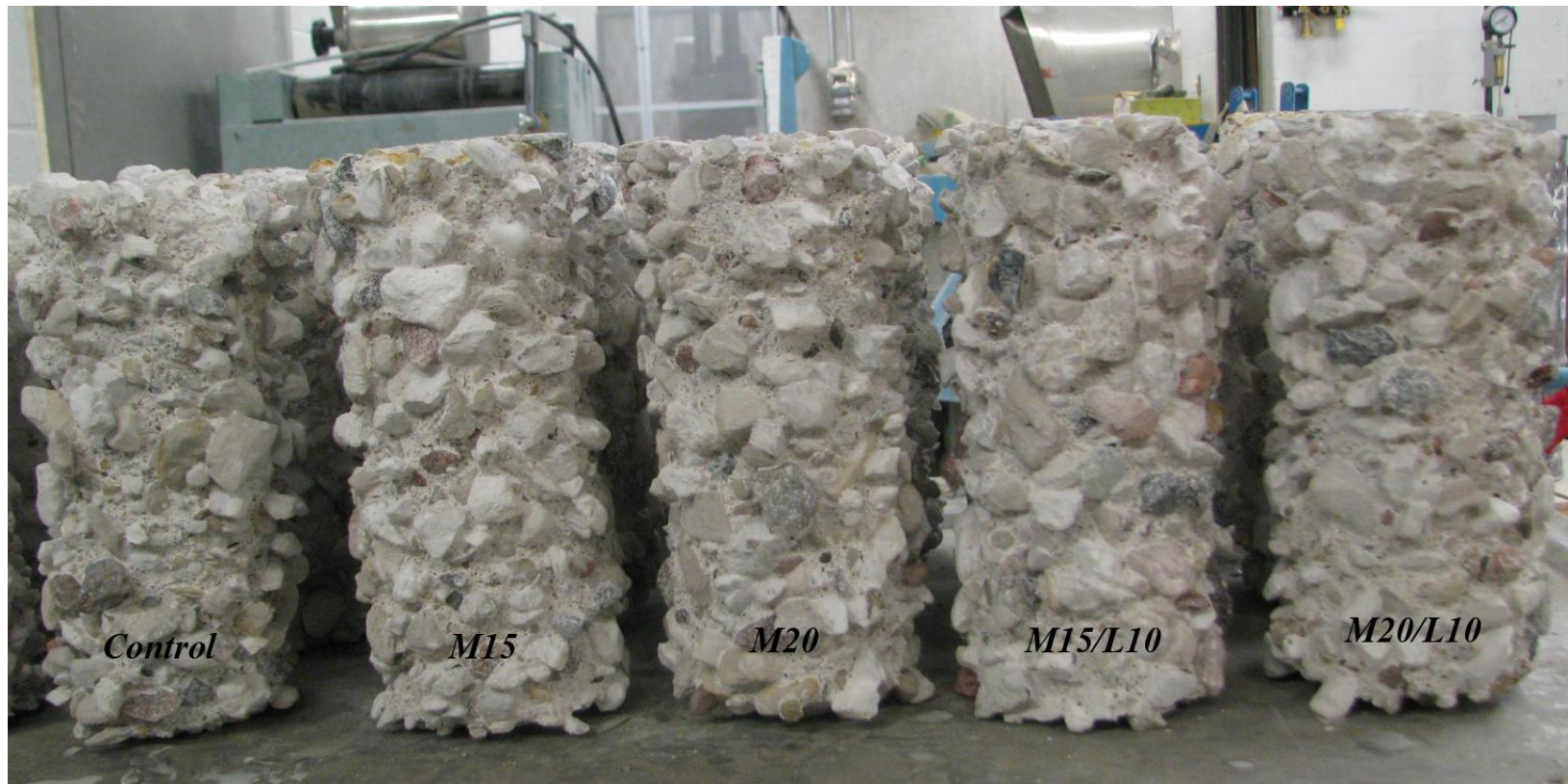
Concrete specimens immersed in 7% sulfuric acid solution for the period of 6 weeks
