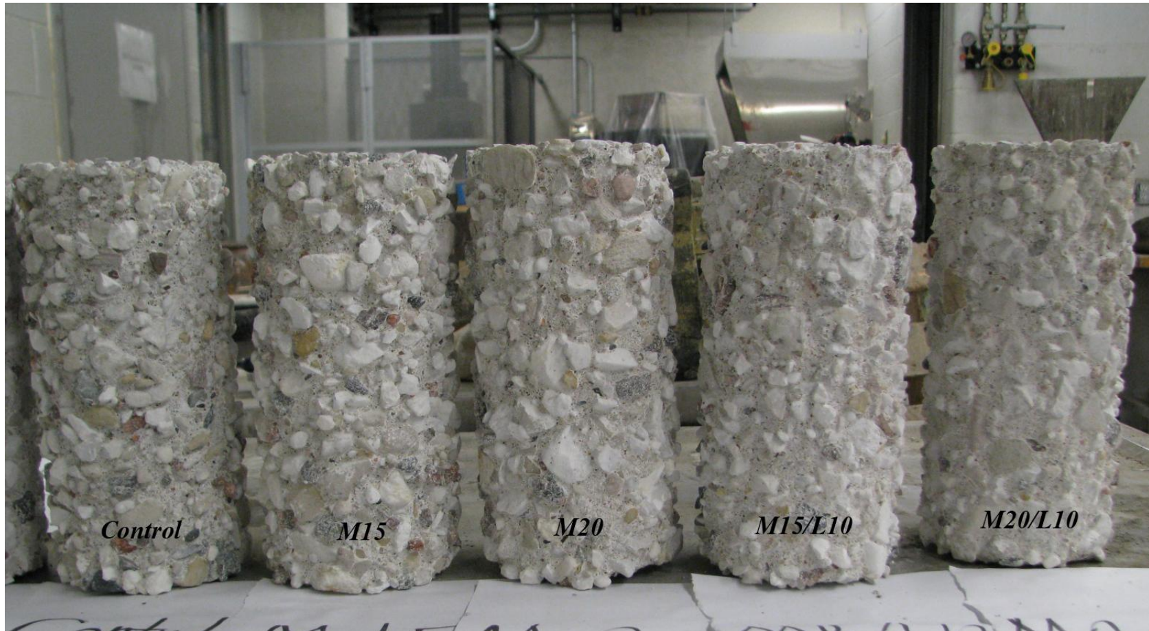
Concrete specimens immersed in 7% sulfuric acid solution for the period of 2 weeks
