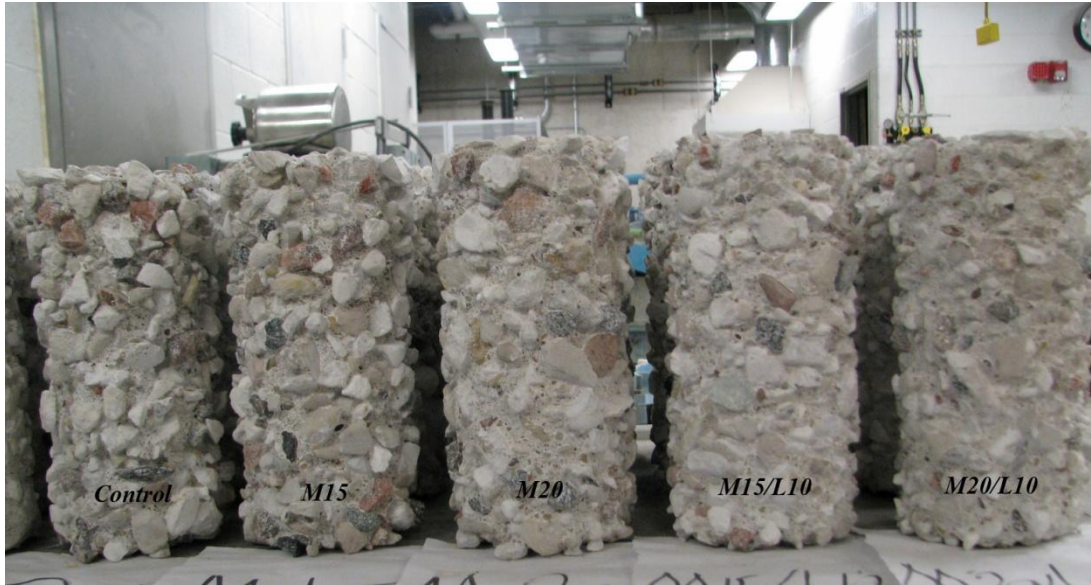
Figure 4.12 Visual assessment of degraded concrete samples after 4 weeks of exposure to a 7% sulphuric acid solution.
