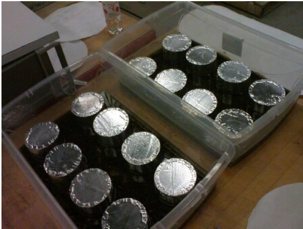
Figure 3.9 Water sorptivity test setup
