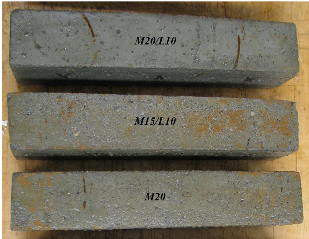
Figure 4.16 Concrete prisms from the M20, M15/L10 and M20/L10 mixes after 300 repeated cycles of freezing and thawing.
