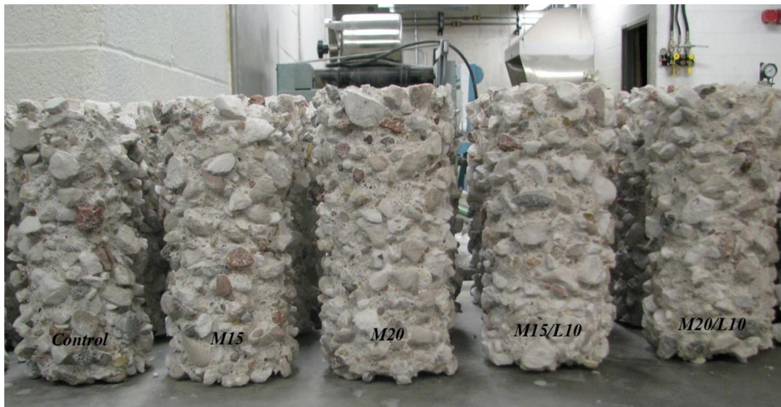
Figure 4.11 Visual assessment of degraded concrete samples after 8 weeks of exposure to a 5% sulfuric acid solution.
