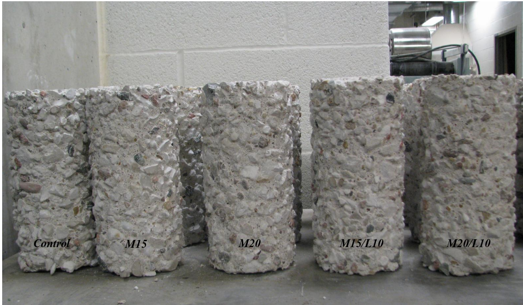
Concrete specimens immersed in 3% sulfuric acid solution for the period of 6 weeks
