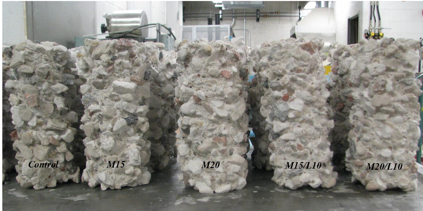
Concrete specimens immersed in 7% sulfuric acid solution for the period of 8 weeks
