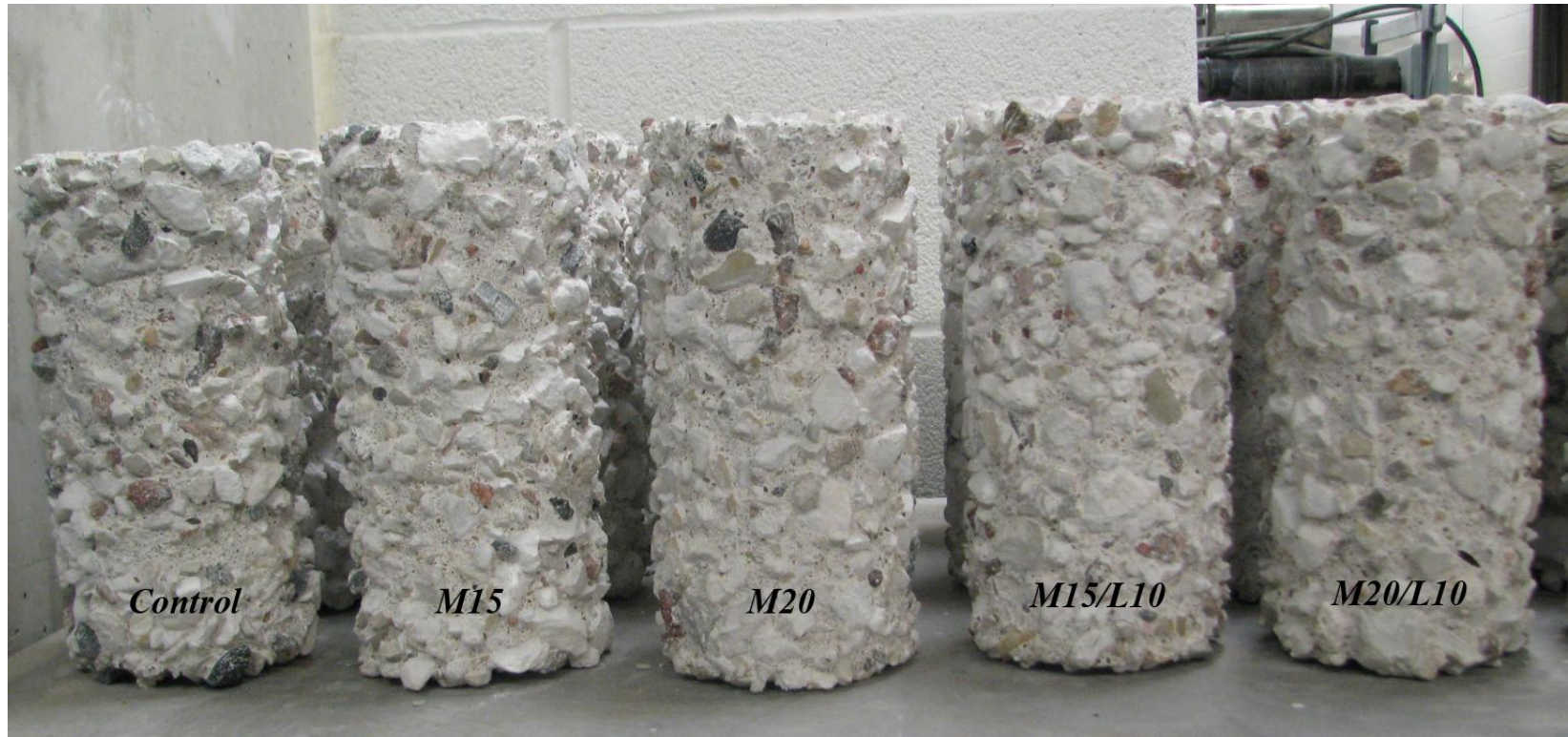
Concrete specimens immersed in 3% sulfuric acid solution for the period of 8 weeks
