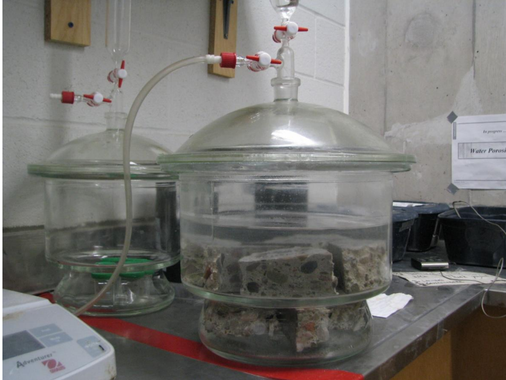
Figure 3.11 The setup of the water porosity test.
