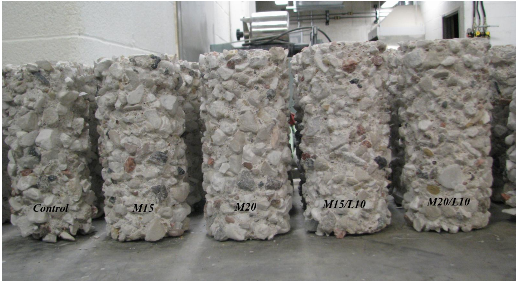
Concrete specimens immersed in 5% sulfuric acid solution for the period of 6 weeks
