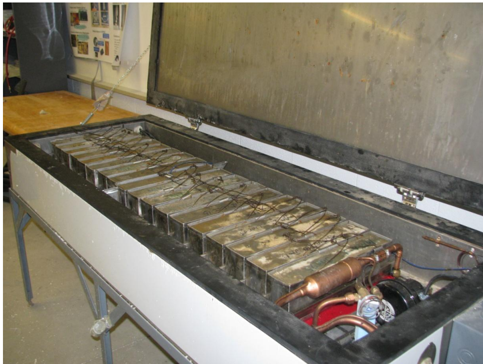
Figure 3.10 Rapid freezing and thawing test setup
