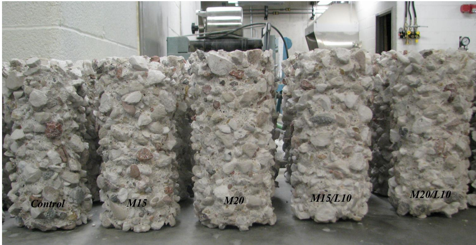
Concrete specimens immersed in 5% sulfuric acid solution for the period of 8 weeks
