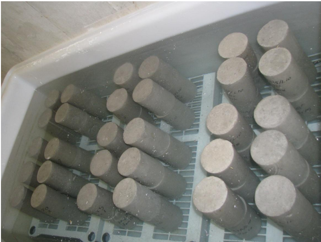
Figure 3.8 Concrete specimens in fresh sulfuric acid solution.
