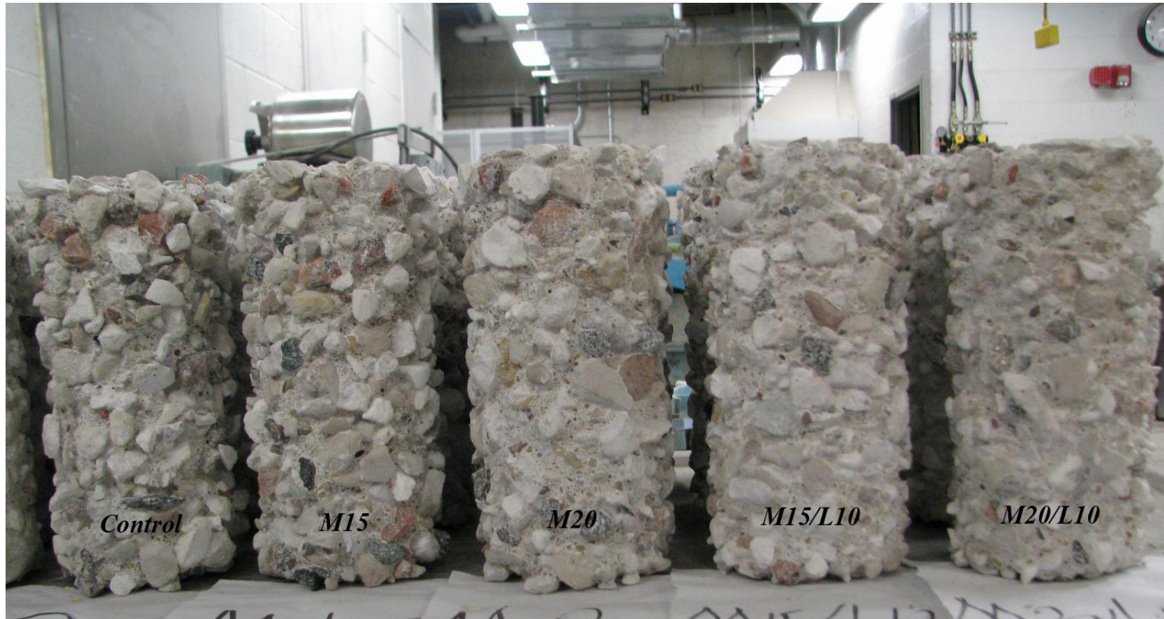
Concrete specimens immersed in 7% sulfuric acid solution for the period of 4 weeks
