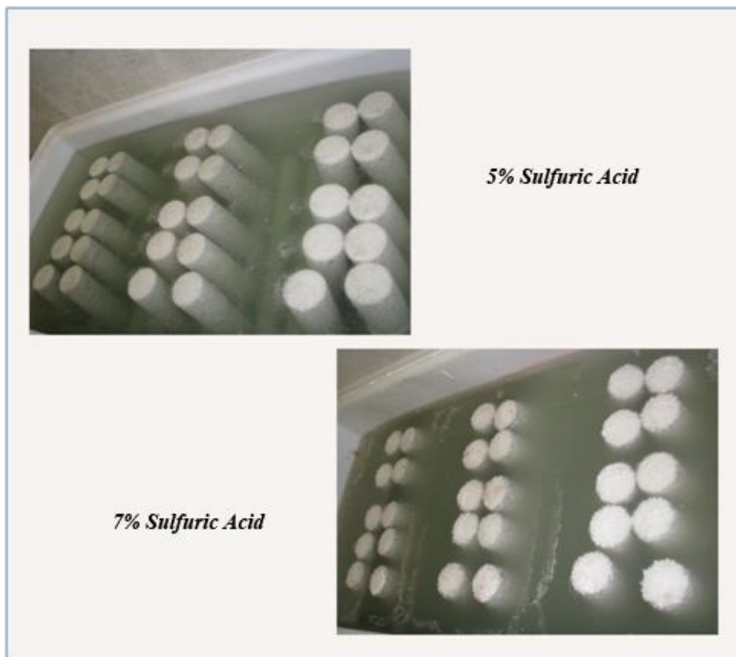
Figure 4.1 Specimens inside the tanks which contain sulfuric acid solutions.
