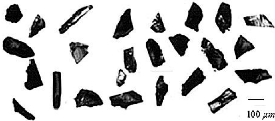
Figure 2.1. Geometry of 90 Grit SiC particles.
