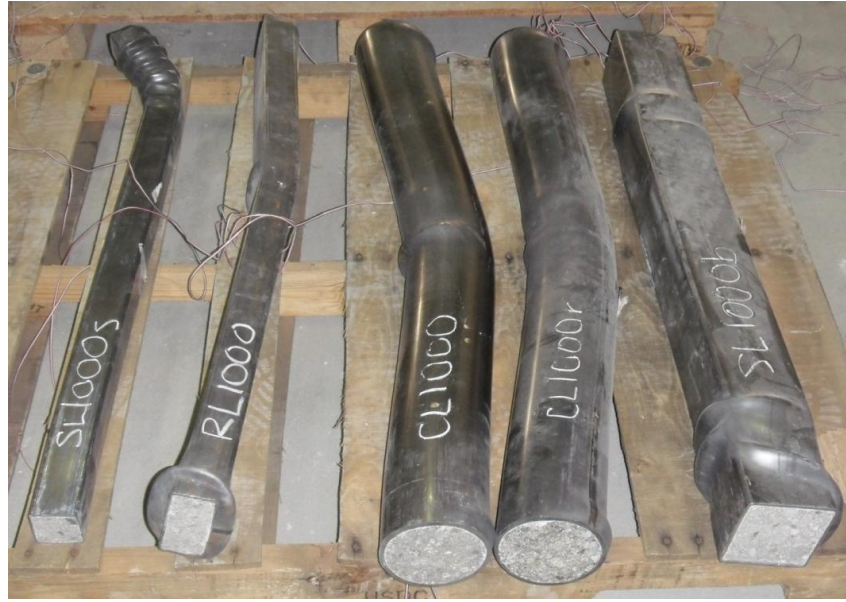
Figure 5.13: Failure modes of LWC-filled CFST columns
