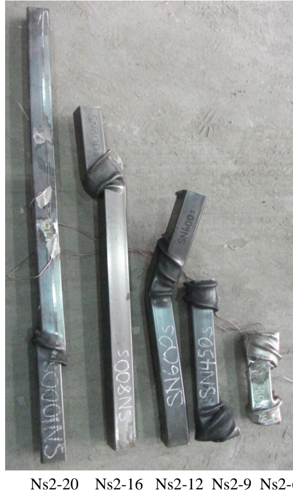
Figure 5.2: Failure modes of NC-filled CFST columns
