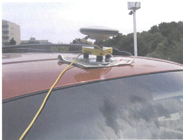
Figure 4.12 Antenna Set-Up for Kinematic Observation
