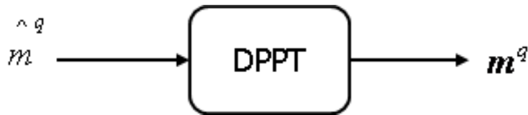
Figure 4.8: DPPT-based TF feature extraction of a signal with linear time-varying frequency.
