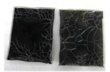
Figure 4.5: Negative Degradation: Vinegar Syndrome Displaying Channelling
