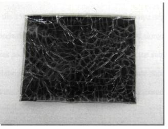
Figure 4.4: Negative Degradation: Vinegar Syndrome Displaying Channelling
