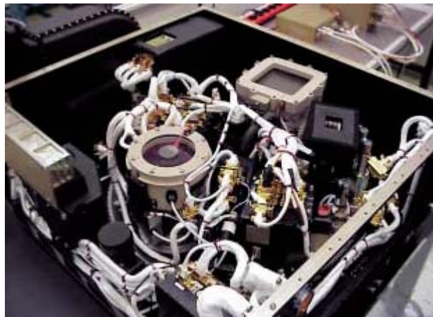
Figure 2-9 The three Experiment Containers installed on FluidPac's rotating carrousel [61].
