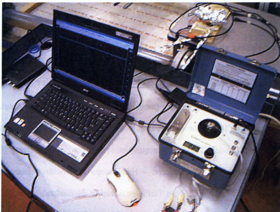
Figure E.1-1 Calibration setup for bi-axial accelerometer for cantilever cylinder in one axis
