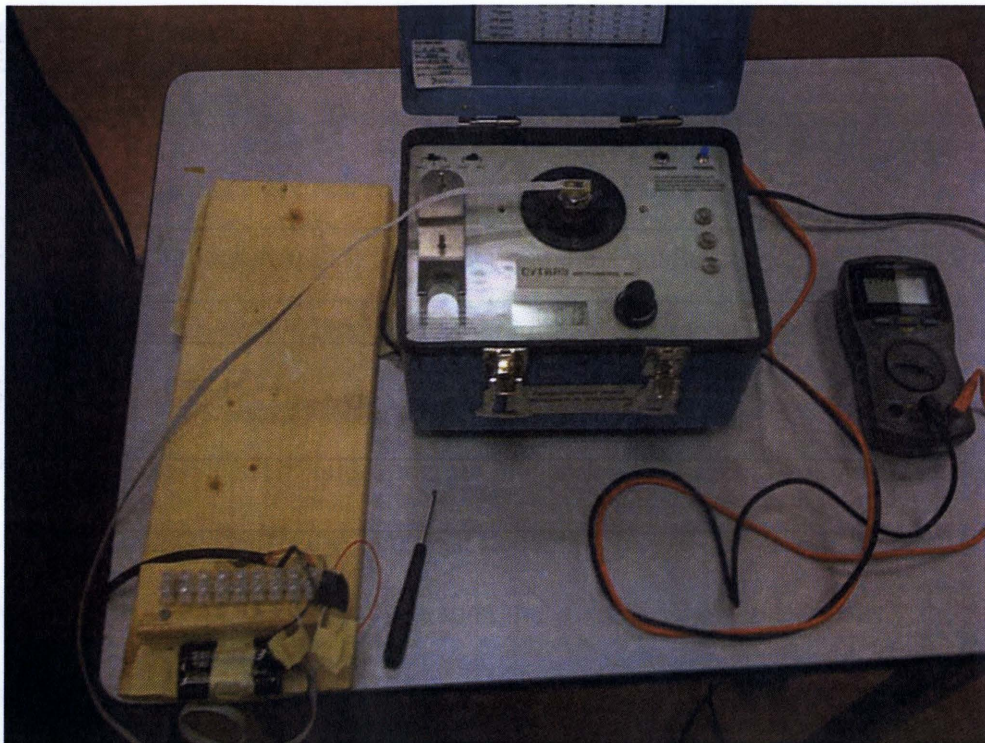
Figure E.2-2 Close-up view of calibration of tri-axial accelerometer for cantilever plate in one axis
