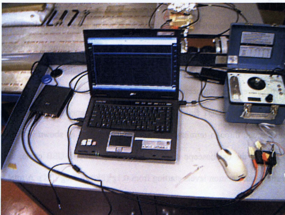
Figure E.1-2 Calibration setup for bi-axial accelerometer for cantilever cylinder in second axis
