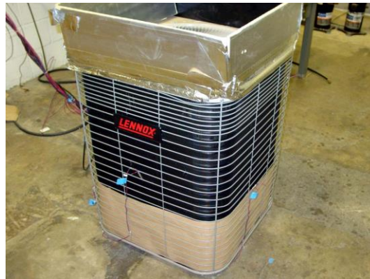
Figure 2-17 Heat pump setup with improper flow fault (Payne et al., 2009)
