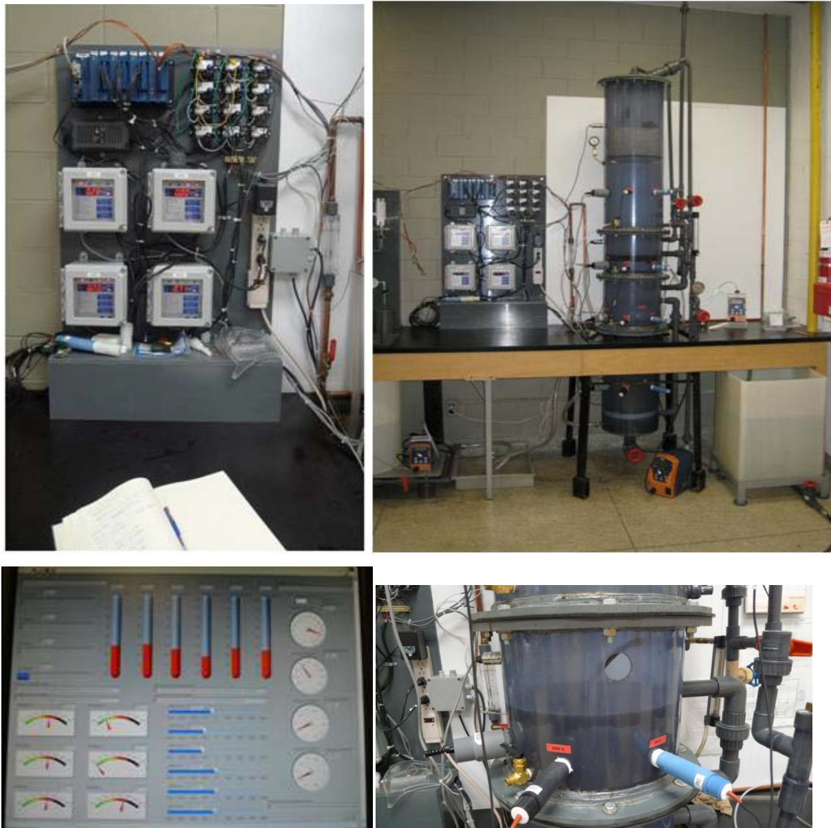
Figure 3.18: CUBEN's pH, ORP and DO Sensors Connected to DAS and Labview Software
