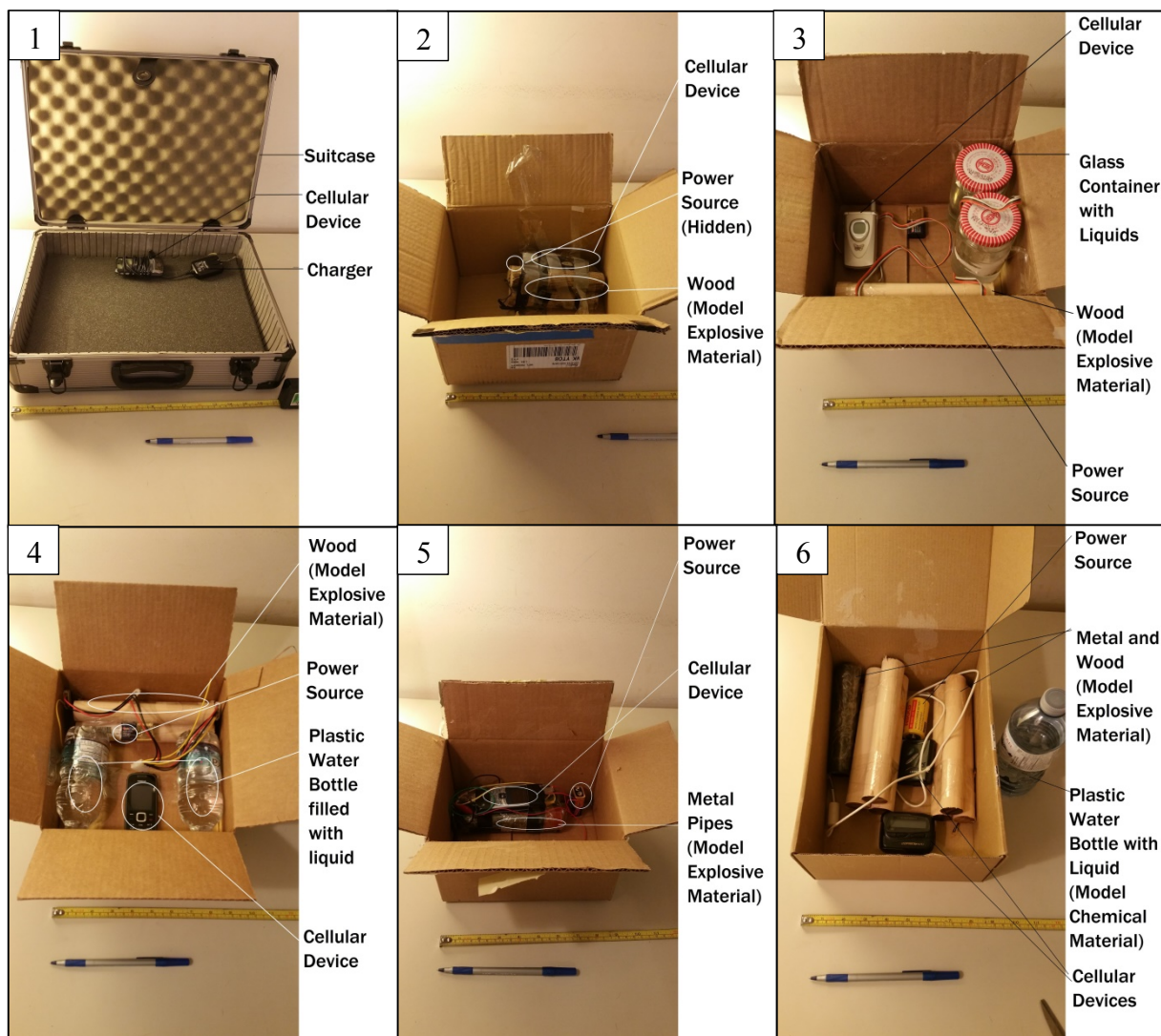
Figure 3.2 – Revealed mock IED components in cardboard containers. 1. Metal/plastic suitcase with a cell phone - 2-6. Cardboard container with IED components with varying types of material (eg. metal, plastic, glass, or wood).
