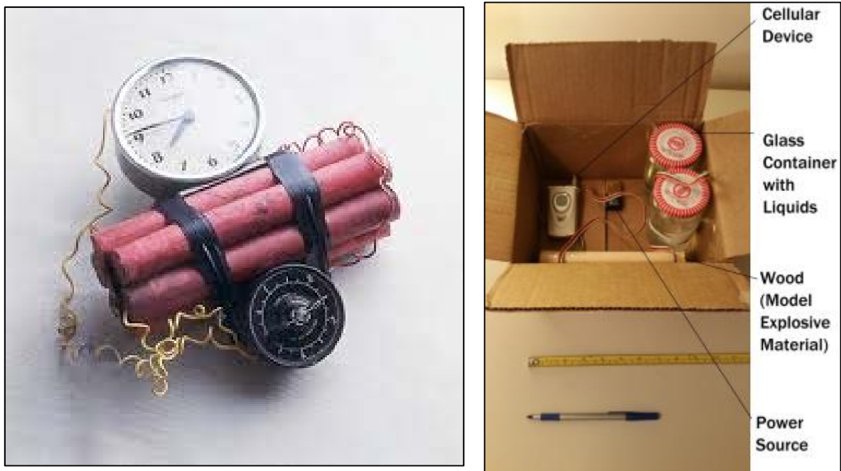
Figure 2.3 - On the left; a real-world IED [29] and on the right, a mock IED. Both share a common set of components and consist of the following: A switch/trigger, a triggering mechanism, main charge (explosive material), a power source for the switch/trigger, and a container.
