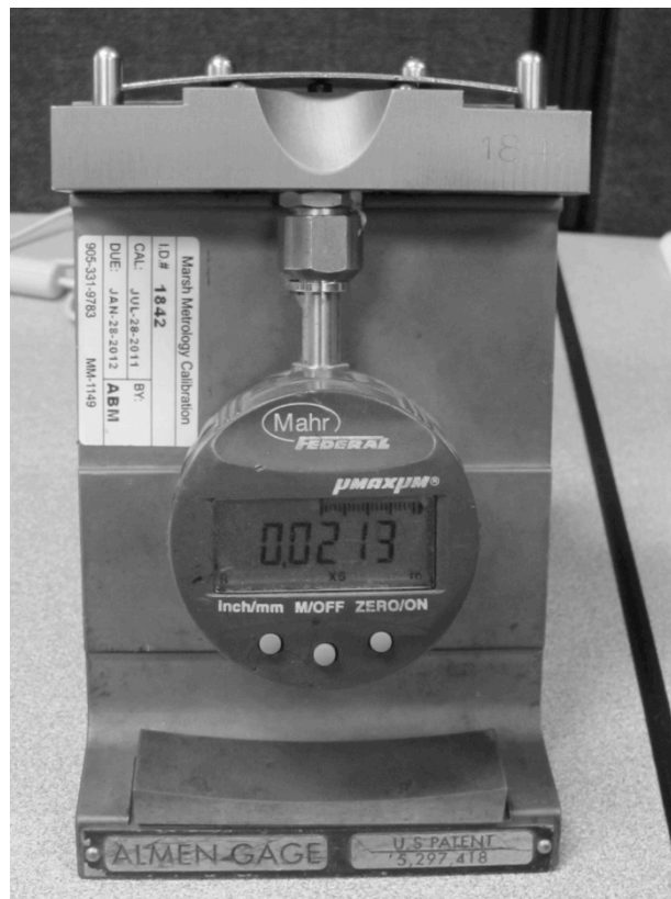
Figure 4-8: Almen Gauge for measuring curvature of Almen strips
