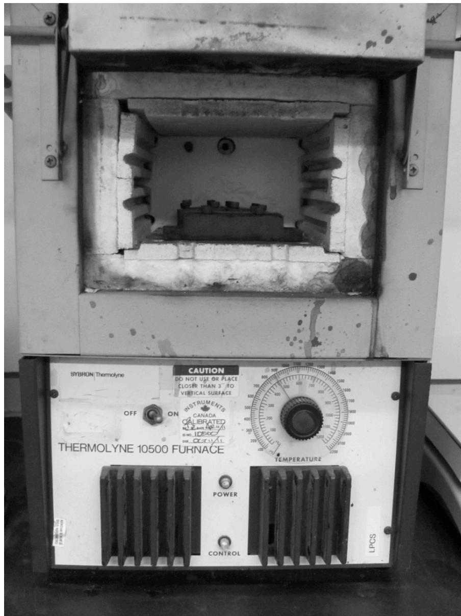
Figure 4-12: Industrial Oven with 300M steel Almen Strips
