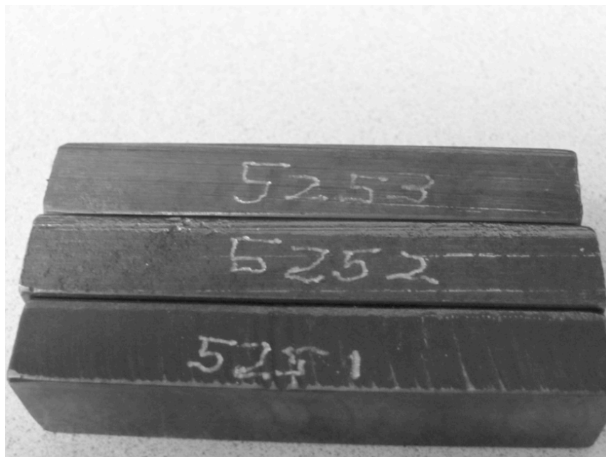
Figure 4-18: Example of vibro-engraving on specimen
