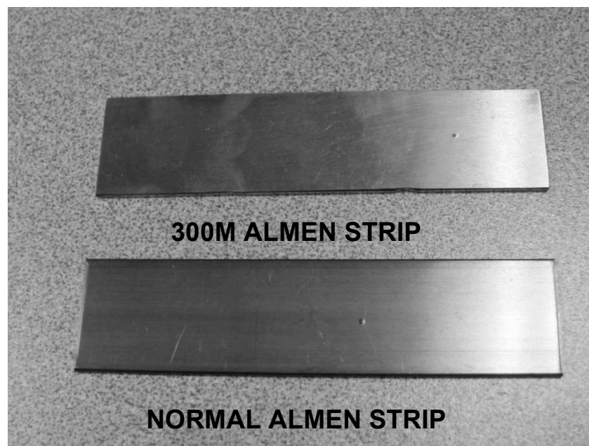
Figure 4-3: Image of 300M steel strip with same dimensions as Almen Strip
