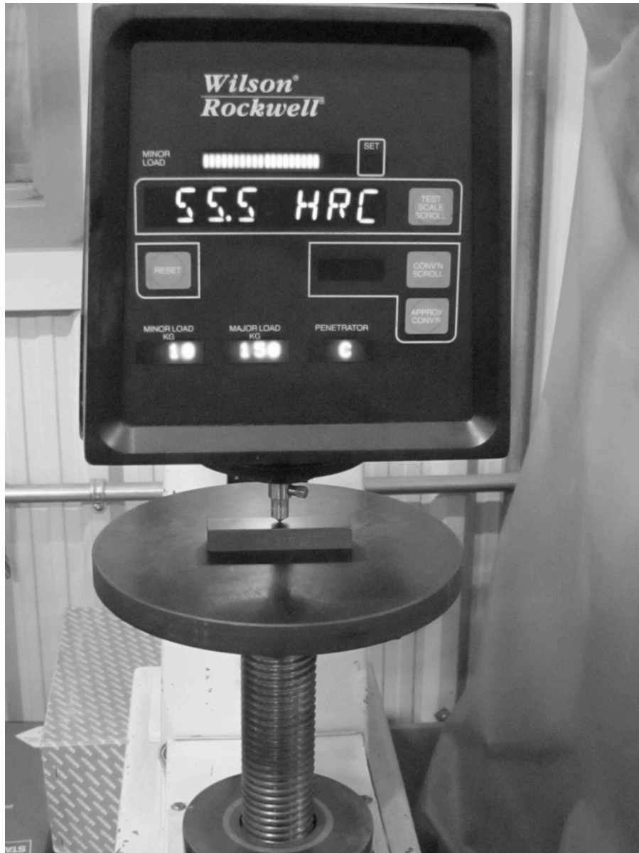
Figure 4-16: Hardness testing machine with specimen
