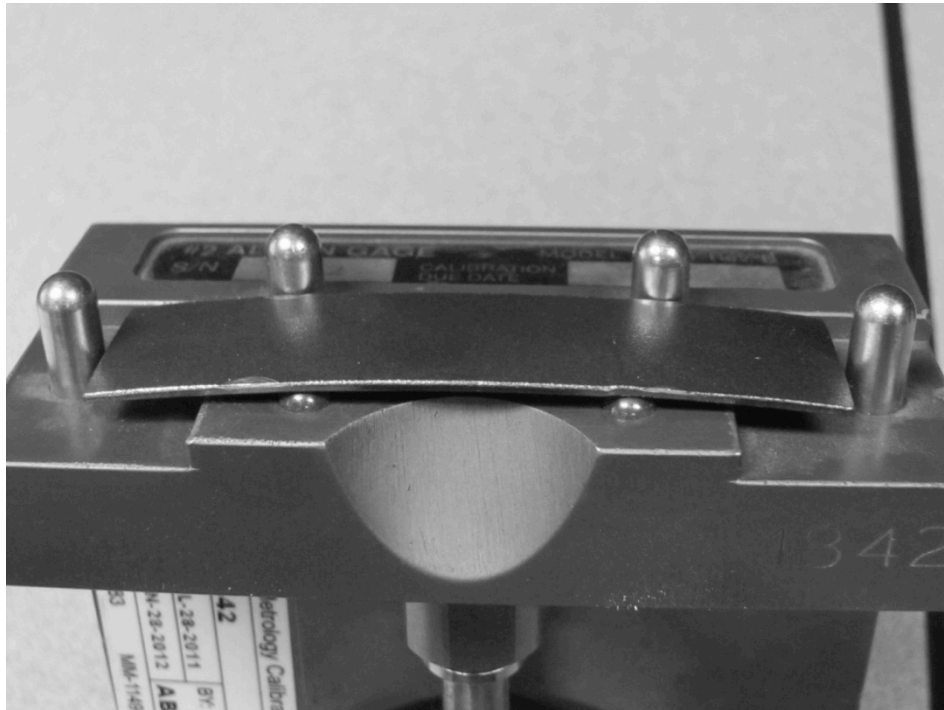
Figure 4-9: Almen Gauge with Almen strip between 4 spindles
