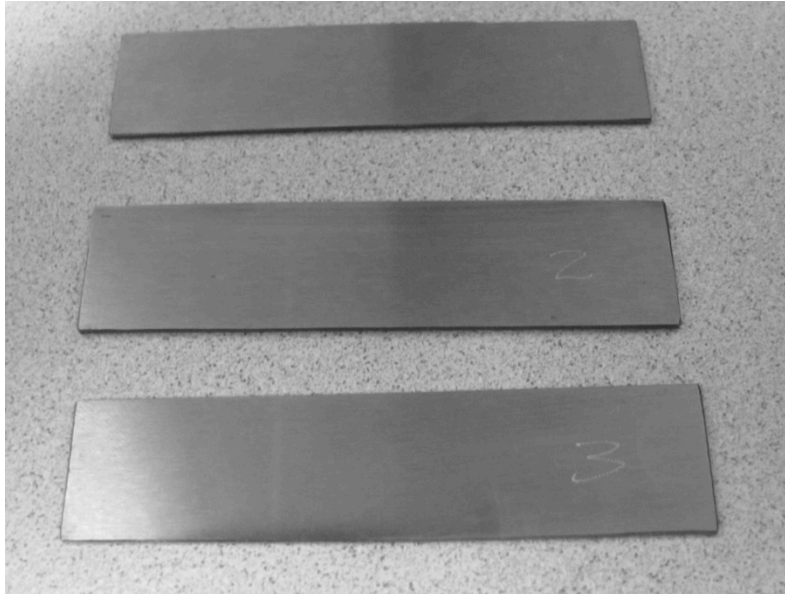
Figure 4-4: Vibro-engraved strip identification
