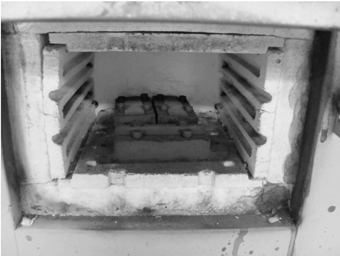
Figure 4-11: 300M steel Almen strips clamped to Almen block during stress relieve
