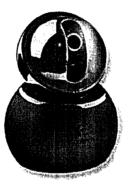
Figure 3.9: Logitech Orbit, NEPWAK's Pan-n-Tilt camera
