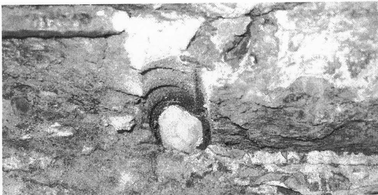
Figure 7-25: SCC-2 Rebar slippage
