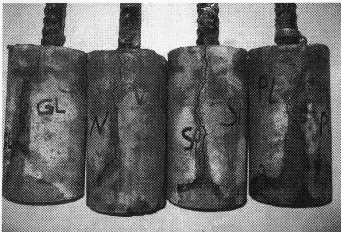
Figure 7-18: Corrosion performance in the small concrete cylinders
