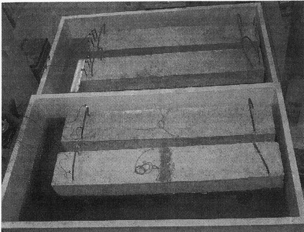
Figure 4-17: Accelerated corrosion tank for corrosion test
