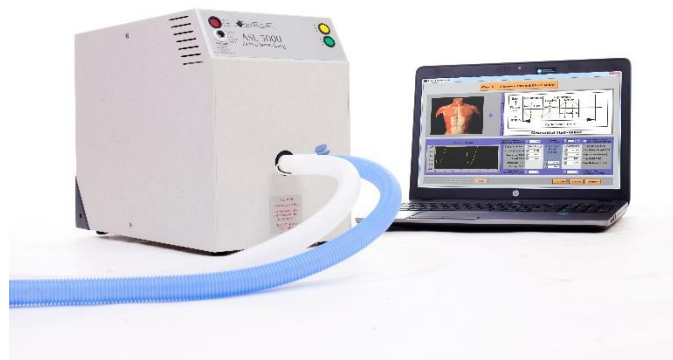
Figure 4.1. The IngMar Medical ASL 5000 (Active Servo Lung). Source: [59]
