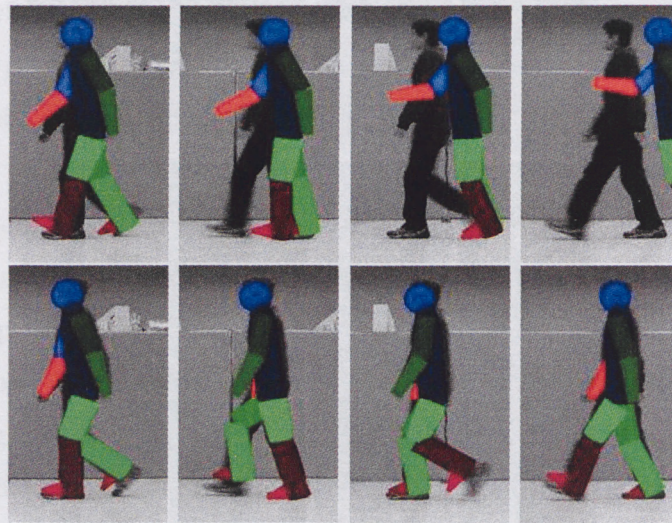
Figure 7.12: Comparison Experiment 4: result before (top) and after (bottom) adopting relative weights for color-cue based measurement function
