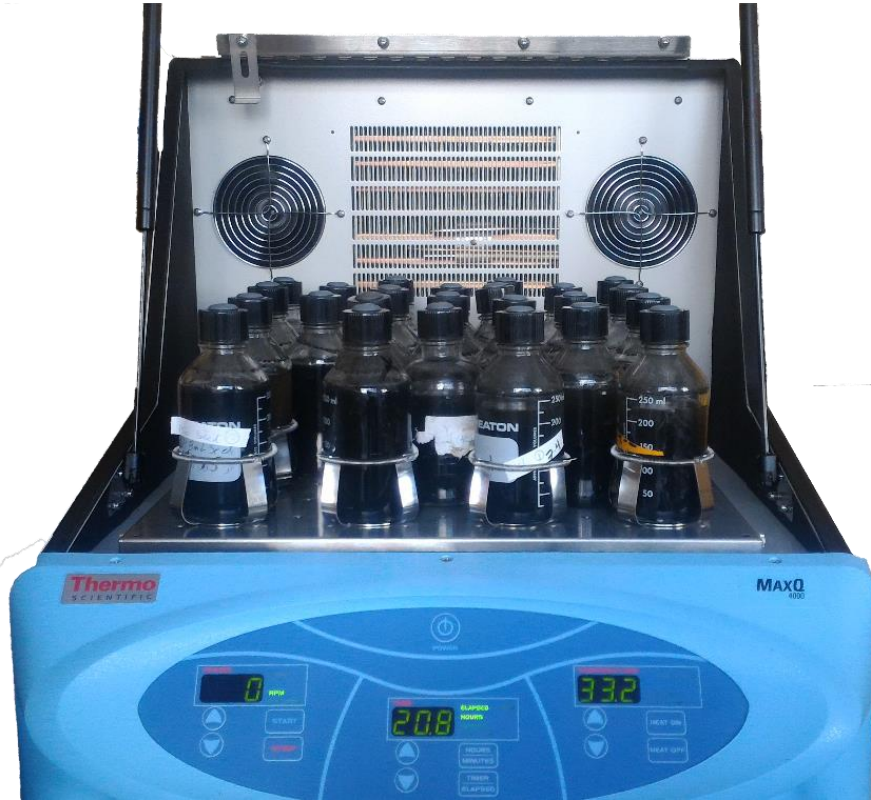
Figure 3-3. Benchtop shaker used for BMP test - Thermo Scientific Benchtop Orbital
