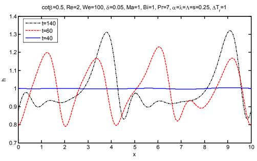
Figure 6.1: Evolution of an Unstable Film Flow
