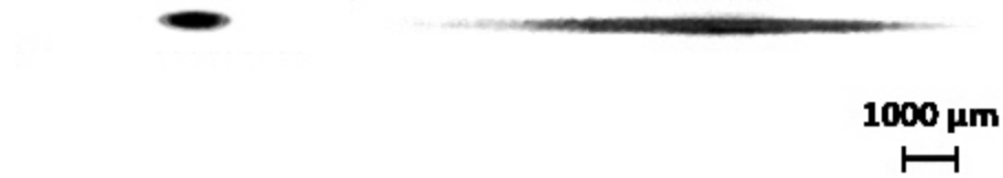
Fig. 2.19 Footprints of the erodent jets produced using the crossed shadow mask (left) and the regular mask (right). For the crossed mask, the slot of the top set of masks was in the vertical direction.
