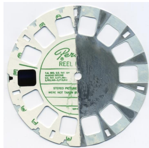
Fig. 5.12 Outer reel layers removed on right to expose aluminium spider Photo by Wolfgang Sell
