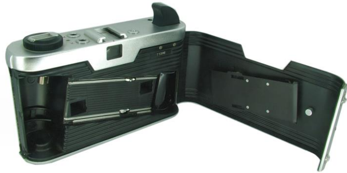
Fig. 5.9 Stereo Color/Mark II diagonal film track Photo by Keith Clatworthy
