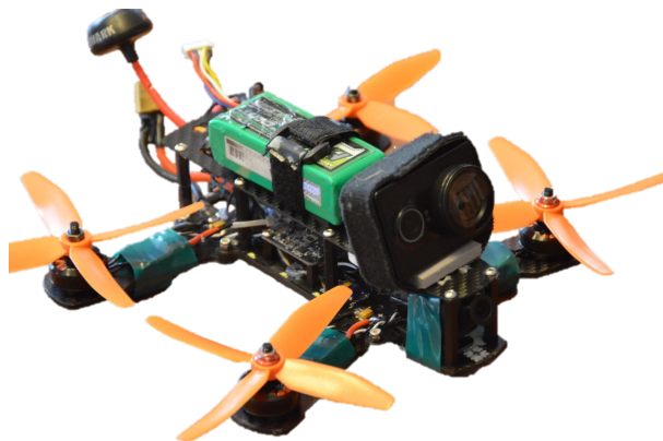
Figure 1.2: Example of a first person view (FPV) racing drone based on the Minion 220 frame by Rotorgeeks [9].
