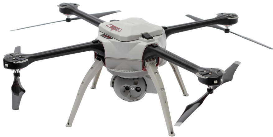
Figure 1.1: Example of a commercial sUAV platform: The Aeryon Labs SkyRanger [3].
