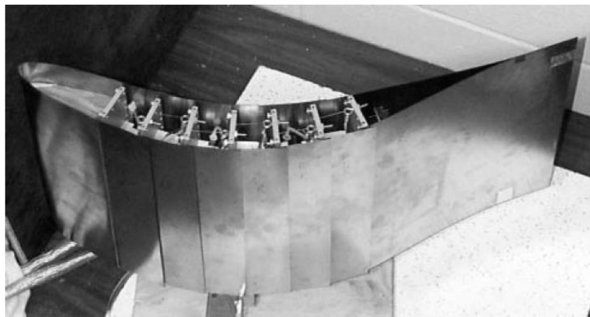
Fig. 9: Hydrofoil under deflection adopted from [47]
