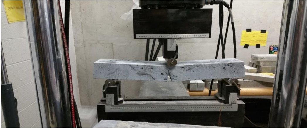
Figure 3.8: Fracture Energy Test Setup and Failed Notched Beam Specimen
