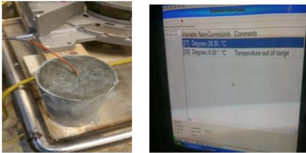
Figure 3.3: Sample and Set up of Time-Temperature Curve Test
