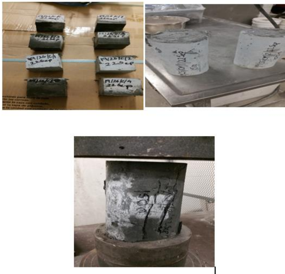
Figure 3.4: Compressive Strength Test on Cylinder and Cube Sample as per ASTM Standard
