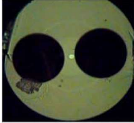
Figure 8 – fibers cross section of Kevin P. Chen et al. experiment [7]
