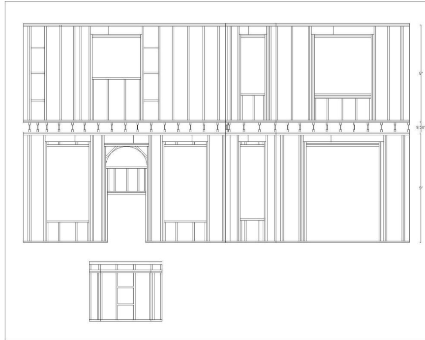
Figure 4.5: Detached house DH4 back-side (north) elevation with the as- built studs installed on the first and second floors including the rim joist area.
