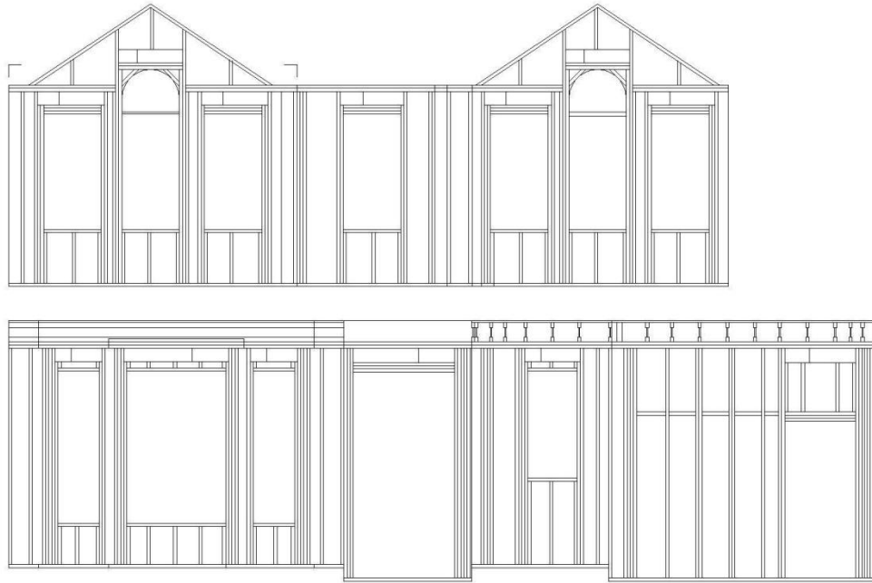
Detached house DH1 front (extended) elevation with the as-built studs
