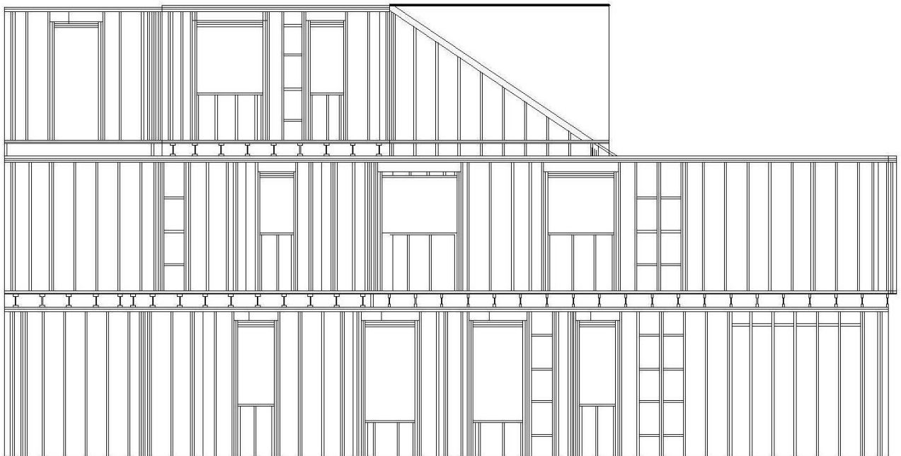
Semi-detached house DH7 east-side elevation with the as-built studs
