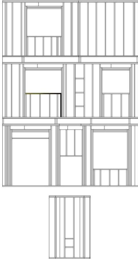
Semi- detached house SDH7 back-side (north) elevation with the as- built studs
