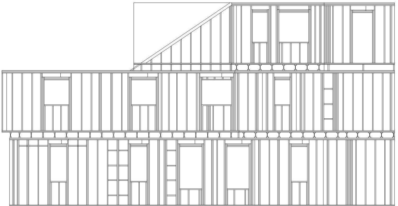
Semi-detached house DH8 east-side elevation with the as-built studs
