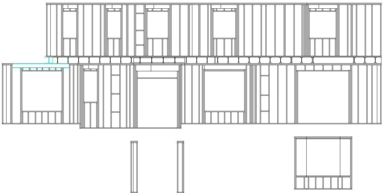
Semi-detached house SDH2 east-side elevation with the as-built studs
