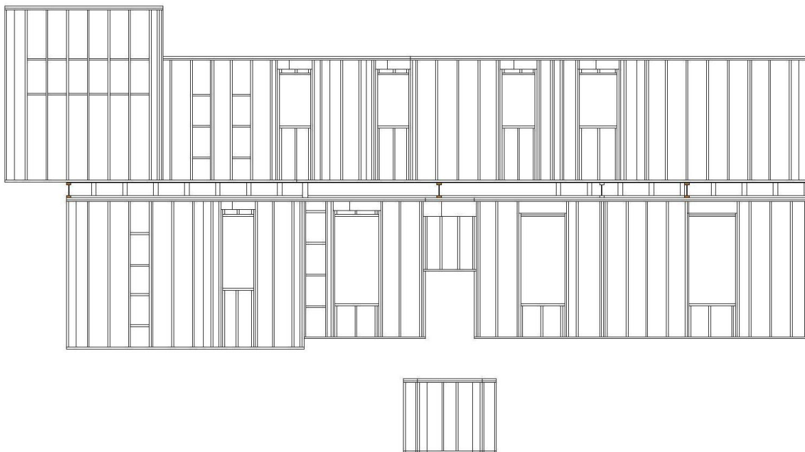
Semi-detached house DH6 east-side elevation with the as-built studs
