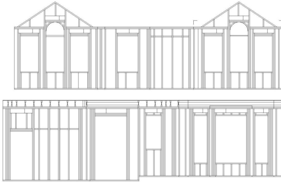
Detached house DH2front (extended) elevation with the as-built studs
