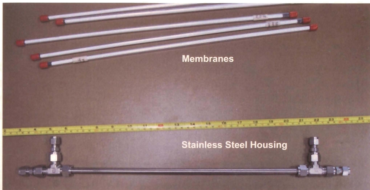
Figure 6.4 Photograph of the ceramic membranes (top) in plastic cases to protect membranes and the stainless steel membrane housing (bottom).
