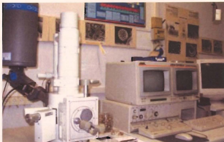
Figure 6.15 SEM and EDS analyzer equipment
