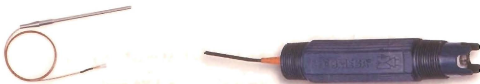
Figure 6.10 Temperature (left) and pH (right) sensors that are connected to the data acquisition system
