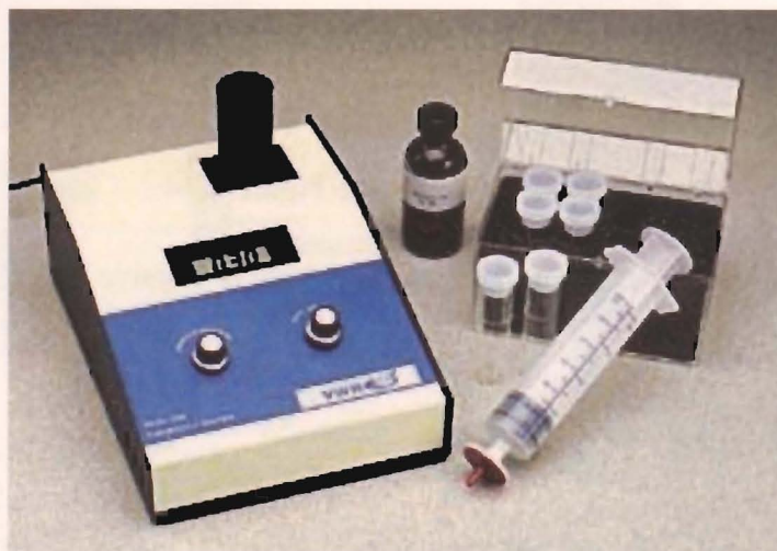
Figure 6.12 VWR® Model 800 Turbidity Meter
