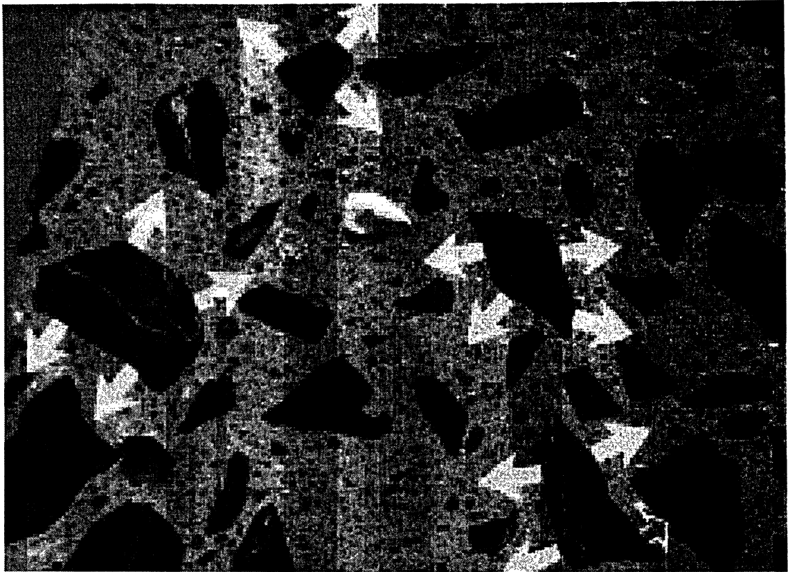
Figure 6: Illustration of expansion forces induced by expanding alkali-silica reactive siliceous limestone particles causing cracking of the particles and the surrounding cement paste (Fournier & Berube, 2000).
