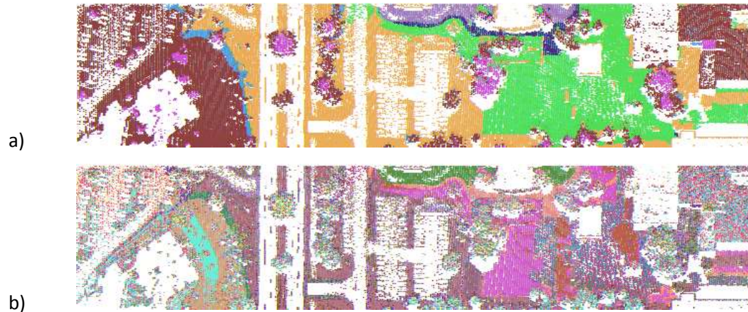
Figure 4-37: Segments of the Multiple-Segments Separation Method a) Segments of the elevation data, b) sub-segments of intensity data
