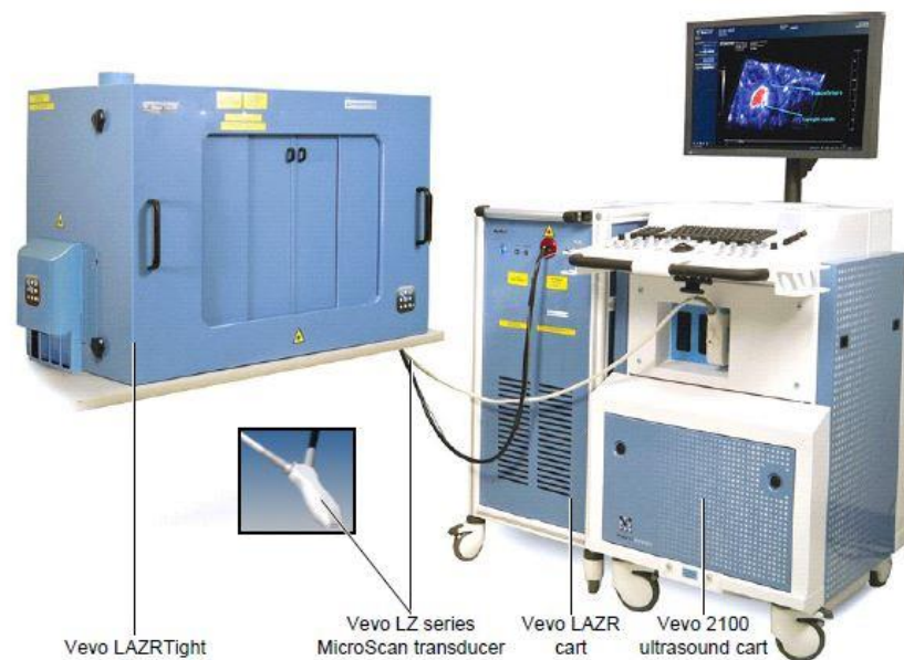
Figure 2-3: The Vevo LAZR Photoacoustic imaging system. The four main components of the imaging system are the Vevo LAZRTight, LZ series transducer, Vevo LAZR cart and the Vevo 2100 US cart with the monitor.
