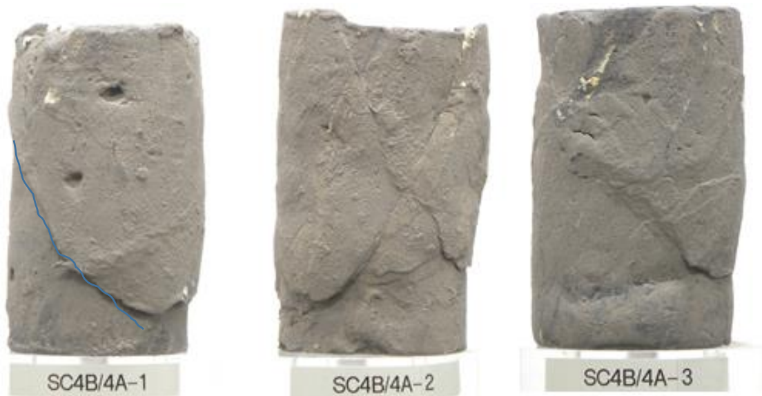
Figure 4-13 The triaxial test result showing different angle of failure in Allen station ( SPL, 2013)
