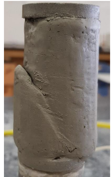
Figure 3-5 Specimen response of normally consolidated clay after shearing (left); Cohesive specimen post-shear showing failure plane (right). (from lab test)
