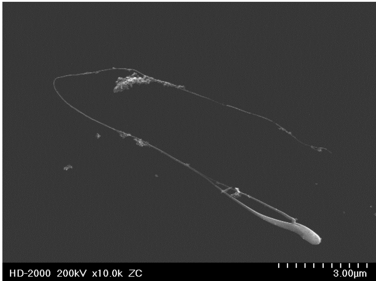
Figure 4–6: Type 3 nanofibers formed by the expulsion of molten droplet
