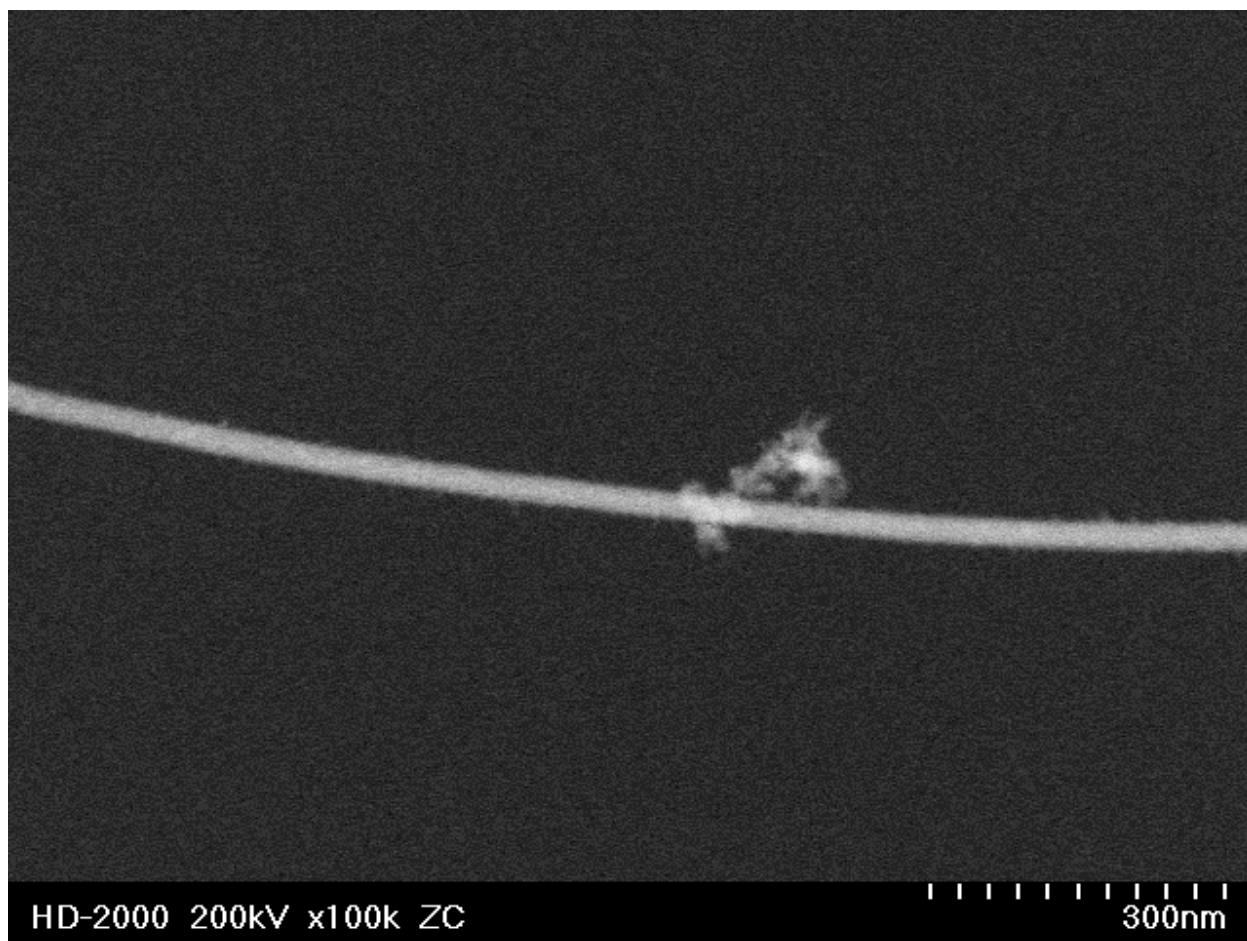
Figure 4-7: Type 4 nanofiber with diameter less than 100 nm
